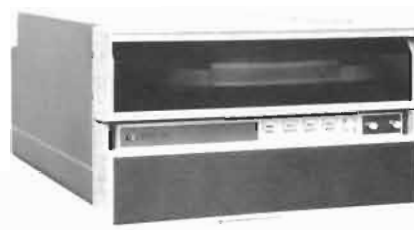
HP Model 7901A has a single removable cartridge disc with a storage capacity of 2.5 million bytes, an average access time of less than 35 milliseconds, and a data transfer rate of 2.5 million bits-per-second. It includes an integral power supply.
