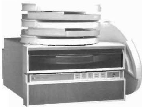
HP Model 7900A has a fixed disc drive plus the removable cartridge for a total storage capacity of 4.9 million bytes, an average access time of less than 30 milliseconds, and a data transfer rate of 2.5 million bits-per-second.
