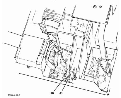
Figure 5-8. PCA Cable Connections
