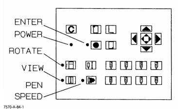
Figure 5-1. Front Panel LEDs
