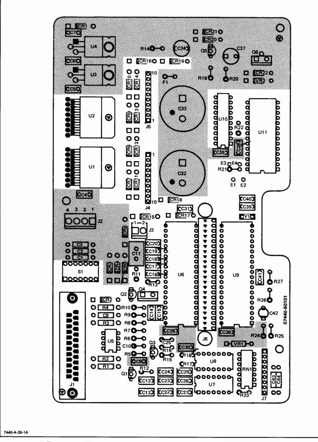
Figure 12-4. HP 7440 Main PCA, Option 001 (RS-232-C), Component Location Diagram
