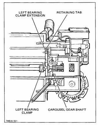
Figure 6-13. Grit Wheel Assembly Removal, Detail A
