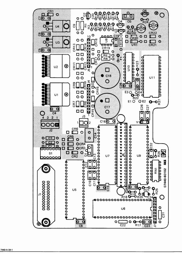
Figure 12-8. HP 7440 Main PCA, Option 002 (HP-IB), Component Location Diagram
