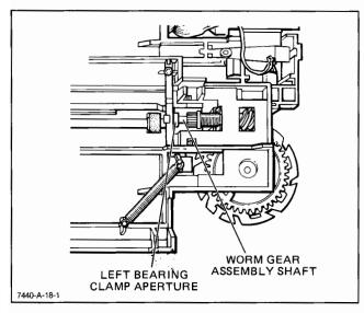
Figure 6-14. Clutch Assembly Removal, Detail F
