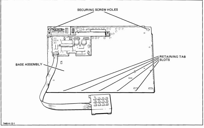
Figure 6-1. Opening up the Plotter, Detail C
