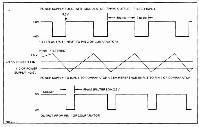
Figure 5-2. Comparator Input and Output Signals
