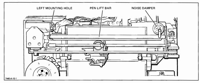
Figure 6-7. Pen Lift Bar Removal, Detail A
