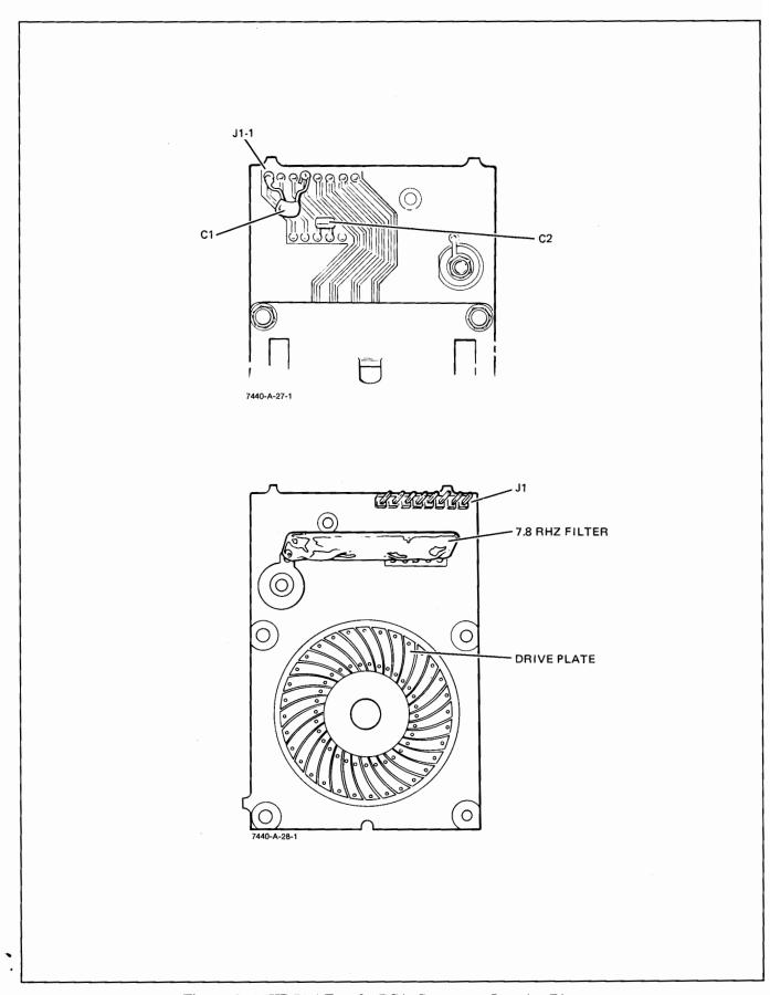
Figure 12-14. HP 7440 Encoder PCA, Component Location Diagram
