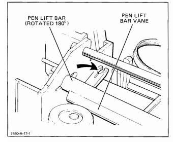
Figure 6-7. Pen Lift Bar Removal, Detail C
