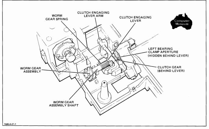
Figure 6-14. Clutch Assembly Removal, Detail E
