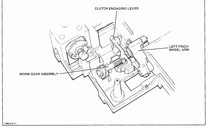
Figure 6-12. Left Pinch Wheel Arm Removal, Detail E
