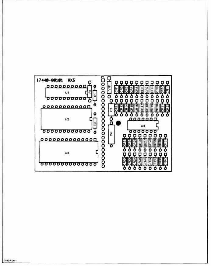
Figure 12-12. HP 17440 Graphics Enhancement Cartridge PCA, Component Location Diagram
