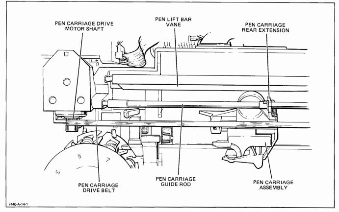
Figure 6-6. Pen Carriage Assembly Removal, Detail B
