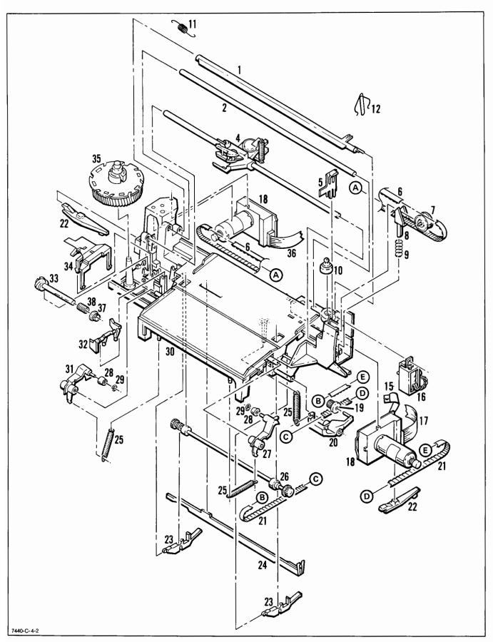
Figure 9-2. Chassis Assembly, Illustrated Parts Breakdown
