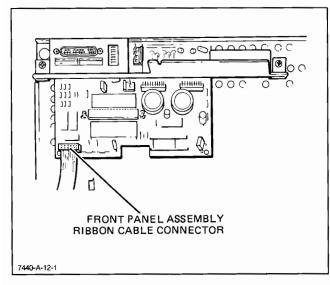
Figure 6-4. Front Panel Assembly Removal, Detail A
