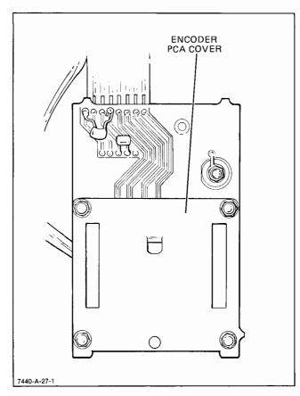
Figure 5-4. Encoder PCA Cover, Outer Side
