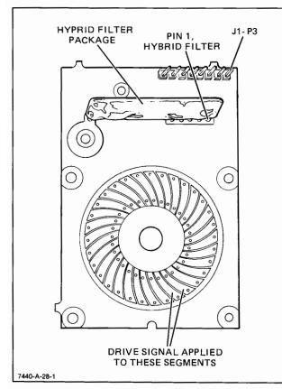
Figure 5-7. Encoder PCA, Inner Side
