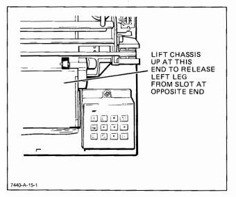
Figure 6-2. Chassis Assembly Removal, Detail C
