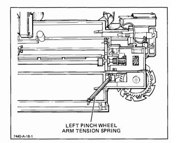
Figure 6-12. Left Pinch Wheel Arm Removal, Detail B
