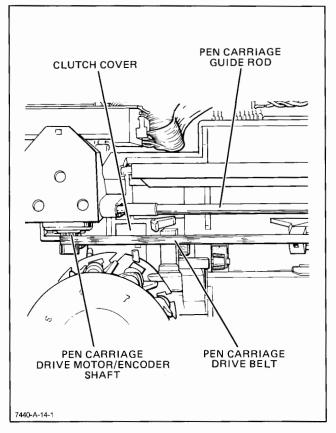
Figure 6-14. Clutch Assembly Removal, Detail C
