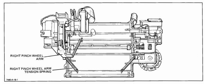
Figure 6-11. Right Pinch Wheel Arm Removal
