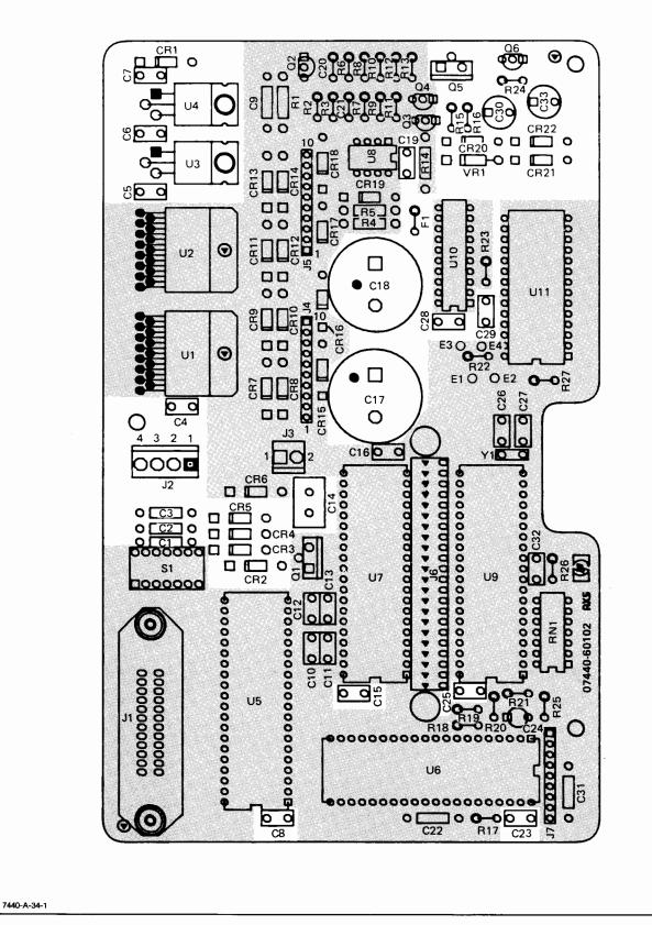
Figure 12-10. HP 7440 Power Supply, Option 002 (HP-IB), Component Location Diagram
