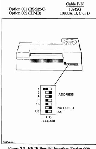
Figure 3-3. HP-IB Parallel Interface (Option 002) **Rear Panel Switch Functions**
