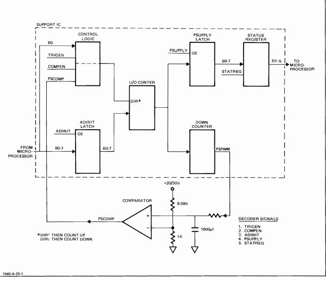
Figure 5-3. Tracking A/D Converter Block Diagram
