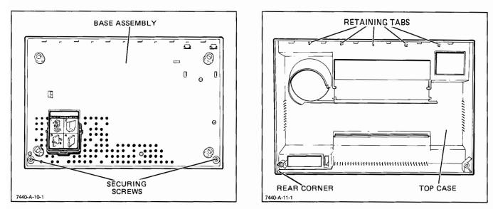
Figure 6-1. Opening up the Plotter, Detail A
