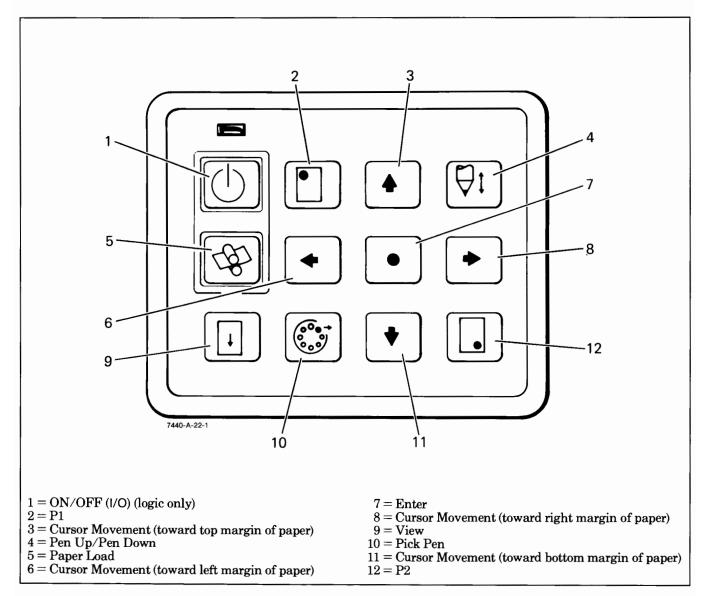
Figure 3-1. Front Panel Key Switches
