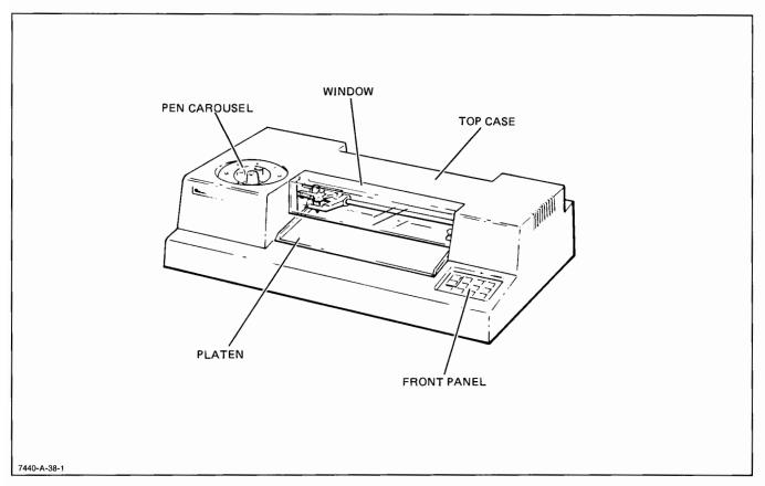
Figure 1-1. HP 7440 ColorPro Plotter, Front View
