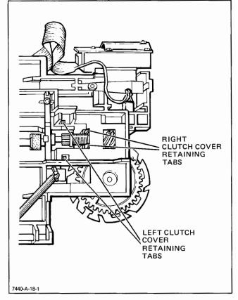
Figure 6-14. Clutch Assembly Removal, Detail D
