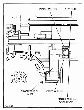
Figure 6-10. Pinch Wheel Removal
