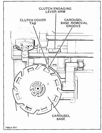
Figure 6-14. Clutch Assembly Removal, Detail A
