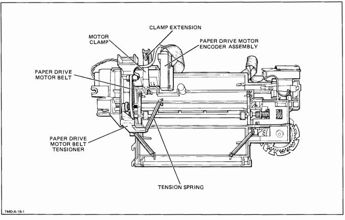
Figure 6-9. Paper Drive Motor/Encoder Assembly Removal
