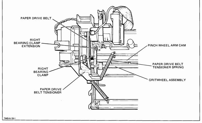
Figure 6-13. Grit Wheel Assembly Removal, Detail B
