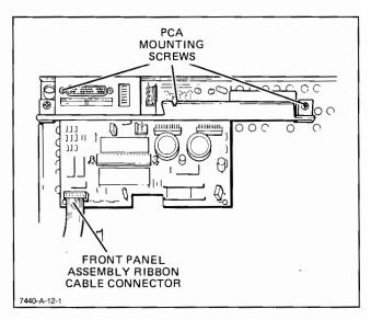
Figure 6-3. Main PCA Removal, Detail A
