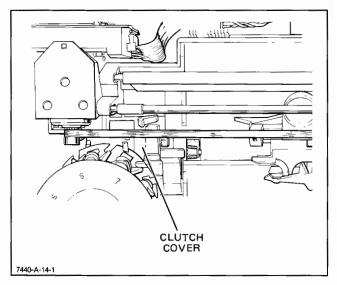
Figure 6-12. Left Pinch Wheel Arm Removal, Detail C
