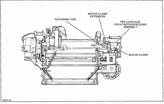
Figure 6-8. Pen Carriage Drive Motor/Encoder Assembly Removal, Detail C
