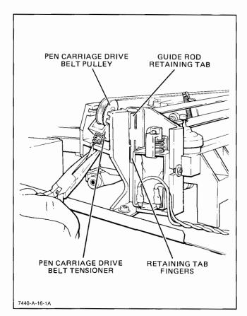
Figure 6-14. Clutch Assembly Removal, Detail B
