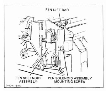
Figure 6-7. Pen Lift Bar Removal, Detail B
