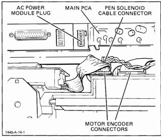
Figure 6-2. Chassis Assembly Removal, Detail B
