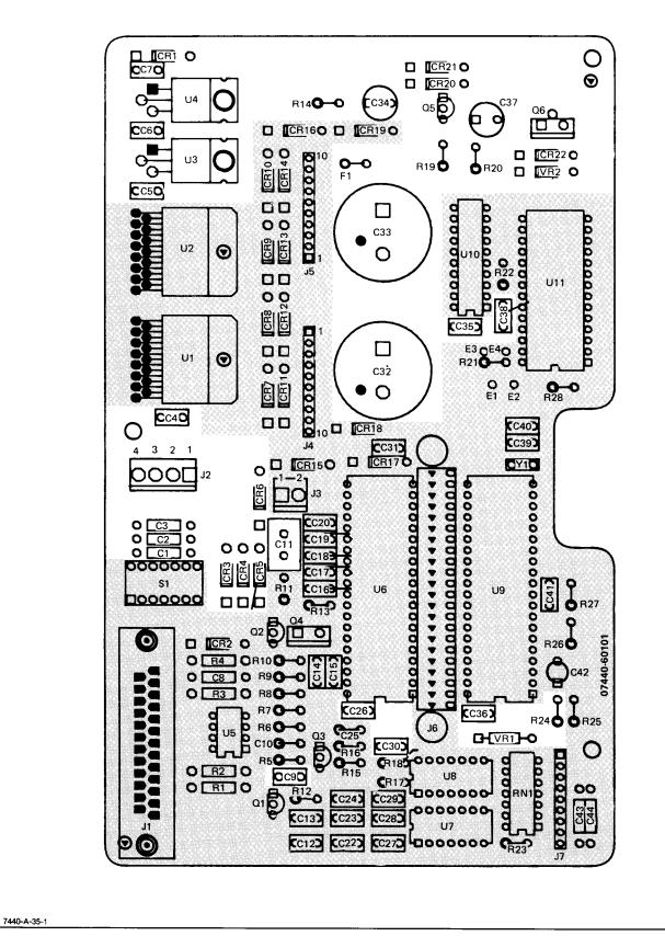
Figure 12-6. HP 7440 Power Supply, Option 001 (RS-232-C), Component Location Diagram
