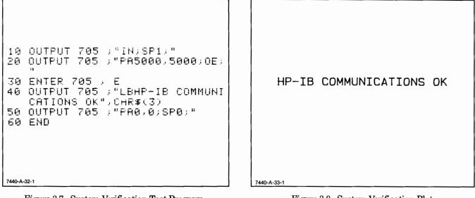
Figure 3-7. System Verification Test Program
