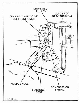
Figure 6-6. Pen Carriage Assembly Removal, Detail A
