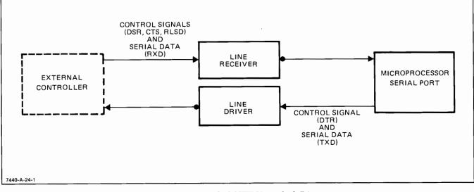
Figure 5-9. RS-232-C/CCITT V.24 Block Diagram
