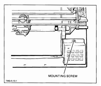
Figure 6-4. Front Panel Assembly Removal, Detail B
