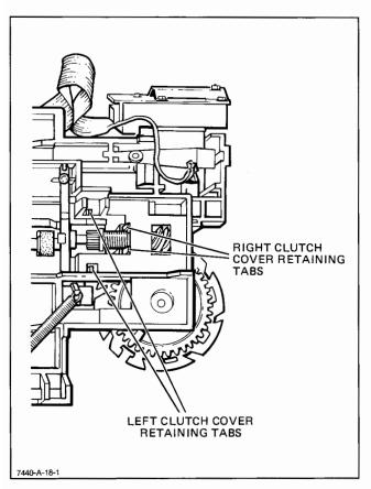
Figure 6-12. Left Pinch Wheel Arm Removal, Detail D
