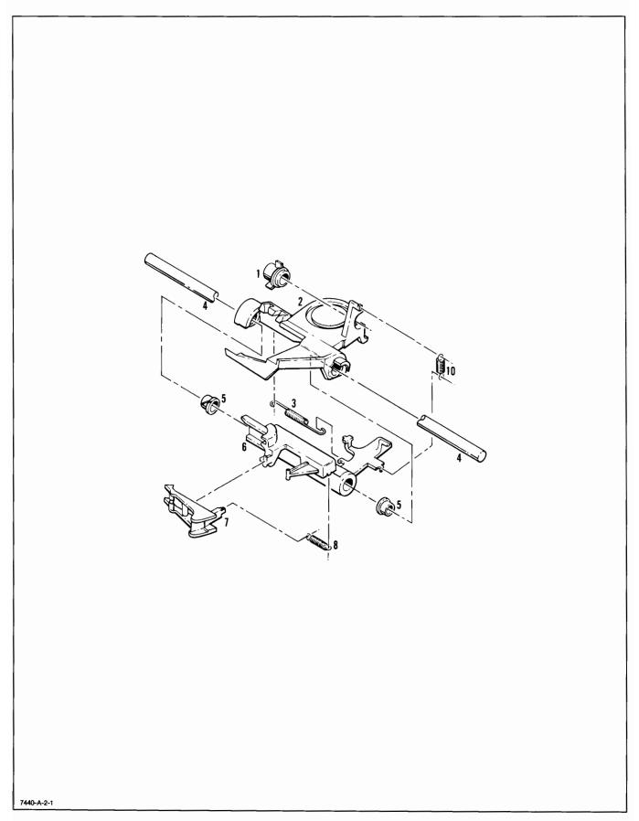
Figure 9-3. Pen Carriage Assembly, Illustrated Parts Breakdown
