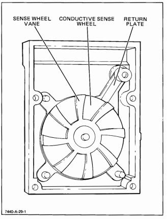
Figure 5-8. Encoder Sense Wheel and Return Plate
