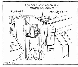
Figure 6-5. Pen Solenoid Assembly Removal, Detail B
