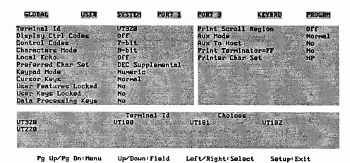
Figure 2-5. System Setup Menu under ANSI Mode
