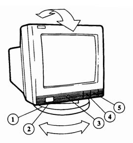
Figure 1-2. Terminal Controls
