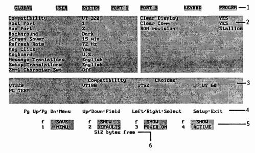
Figure 2-1. Format of Setup Menus
