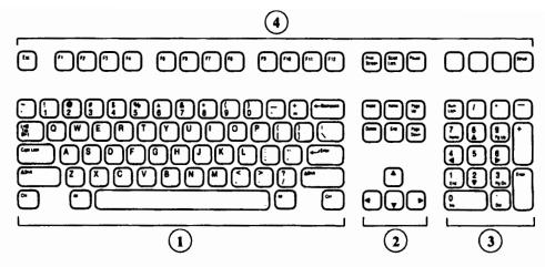
Figure 3-3. The PC-AT Keyboard Layout
