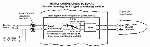
Figure 1. Digital Input Signal Conditioning
