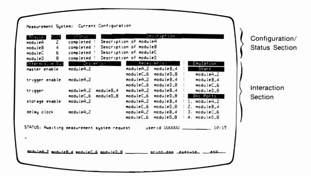
Figure 2-1. Measurement System Display Format
