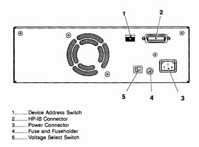
Figure 1-3. The Rear Panel of the 1300H
