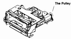
Figure 4-4. Unthreading the tape manually
