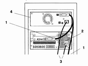
Figure 2-1. Connections to Host and Power
