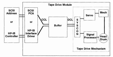
Figure 3-1. The Interface and Tape Drive Module of the 1300H and 1300S
