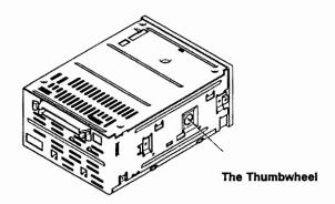
Figure 4-5. Ejecting the cassette manually
