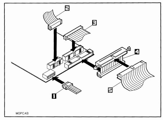
Figure 3-12. Connecting Cables to the Rewritable Optical Controller PCA
