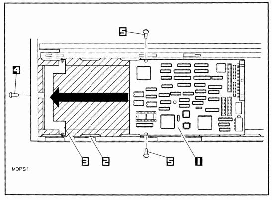
Figure 3-11. Sliding the Rewritable Optical Controller PCA into the PCA Guides
