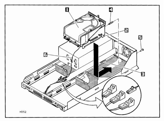
Figure 2-7. Installing the Hard Disk Drive into Slot 2
