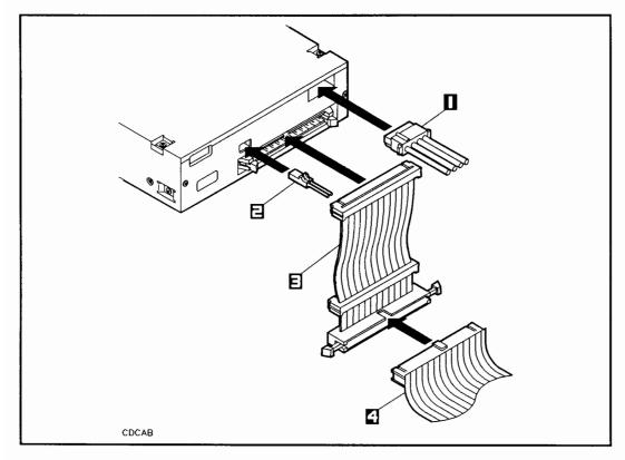
Figure 4-12. Connecting Cables to a CD-ROM Drive
