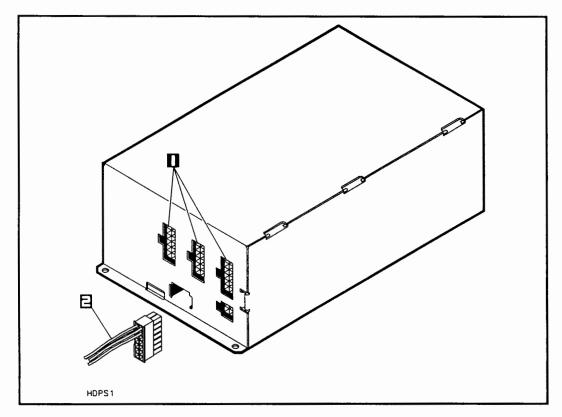
Figure 4-13. Connecting the DC Power Cable
