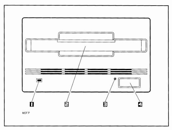
Figure 3-3. Rewritable Optical Disk Drive Front Panel
