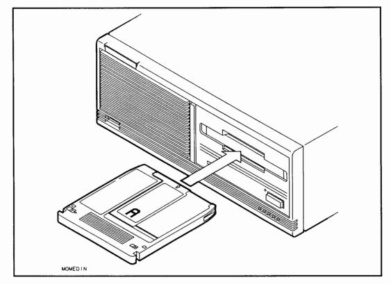
Figure 3-2. Inserting a Rewritable Optical Disk
