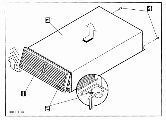
Figure 3-6. Removing the Front Panel and Top Cover
