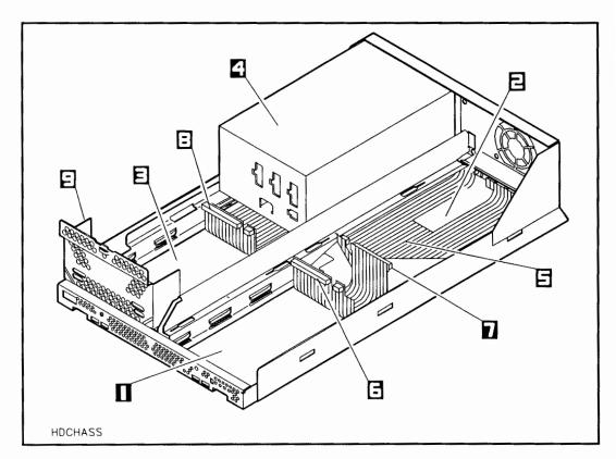
Figure 5-8. Mass Storage System Chassis
