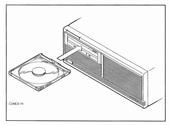
Figure 4-2. Inserting a CD-ROM Disk
