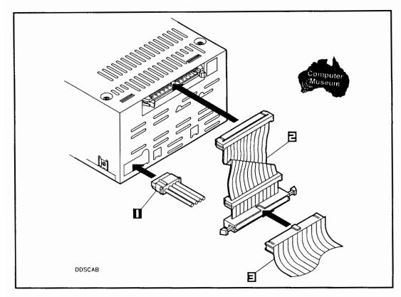
Figure 5-12. Connecting Cables to the DAT Drive
