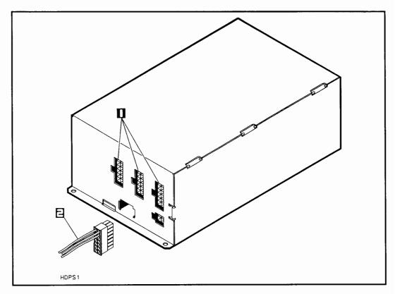
Figure 5-13. Connecting the DC Power Cable
