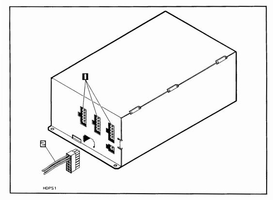
Figure 2-11. Connecting the DC Power Cable
