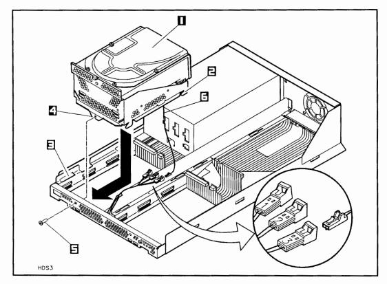
Figure 2-8. Installing the Hard Disk Drive into Slot 3
