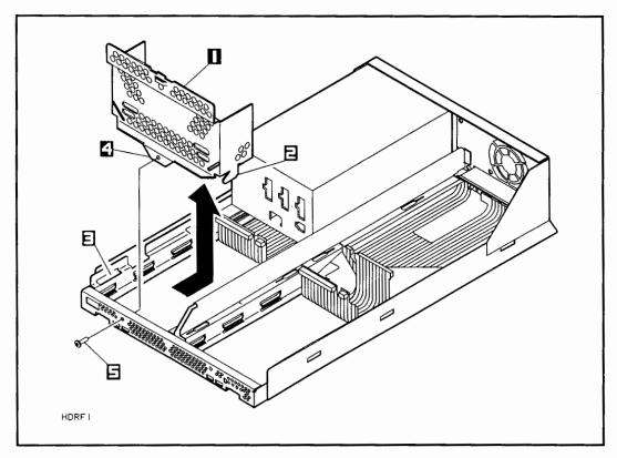
Figure 2-5. Removing the RFI Bracket
