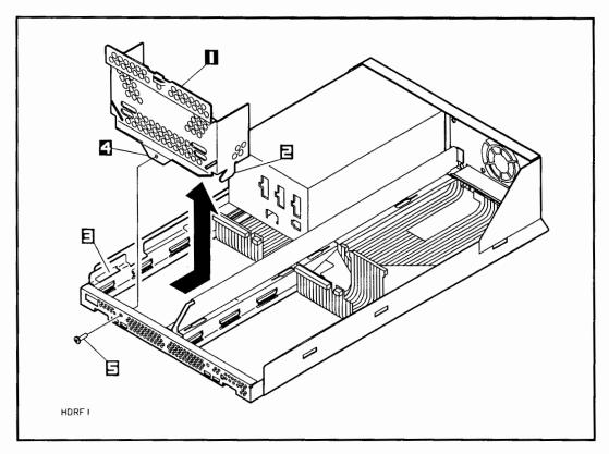
Figure 5-9. Removing the RFI Bracket
