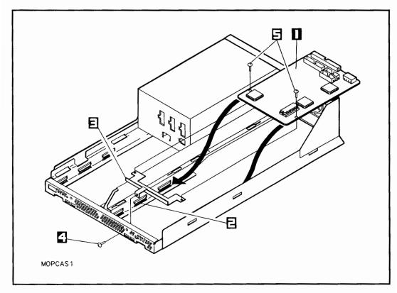
Figure 3-10. Installing the Rewritable Optical Controller PCA
