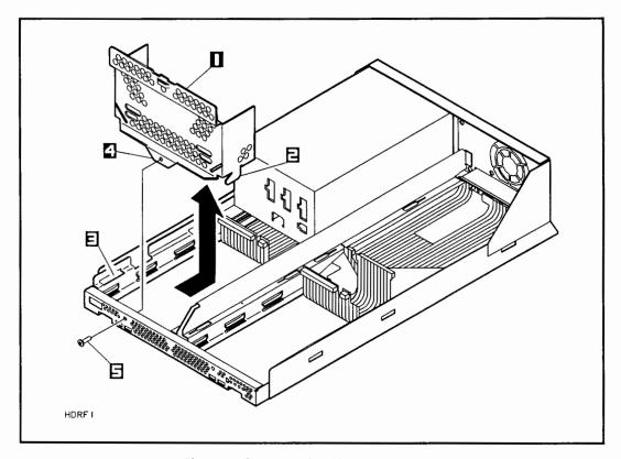
Figure 4-8. Removing the RFI Bracket
