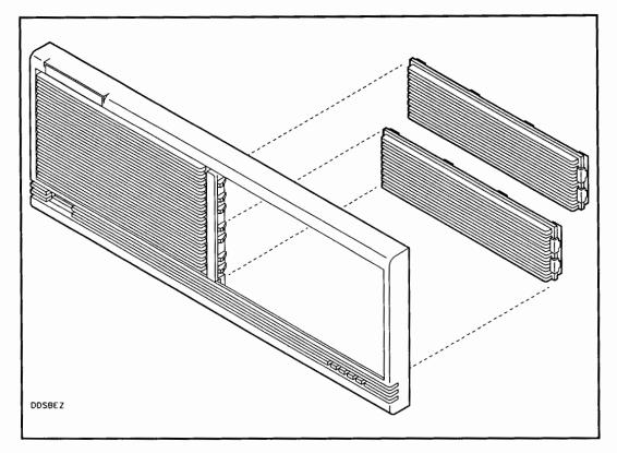
Figure 5-7. Removing the Front Panel Bezels
