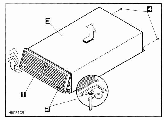
Figure 4-6. Removing the Front Panel and Top Cover
