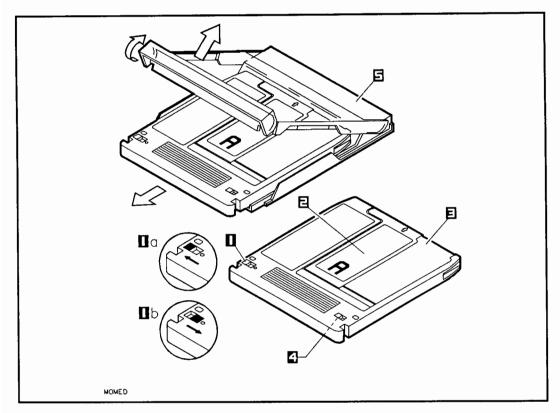
Figure 3-1. Rewritable Optical Disk and Case, Side A
