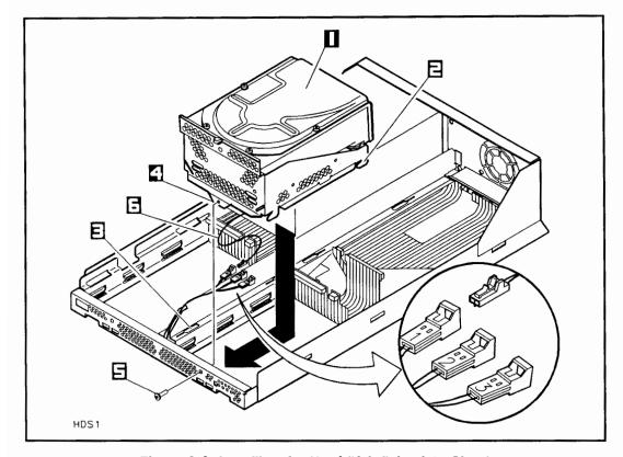
Figure 2-6. Installing the Hard Disk Drive into Slot 1
