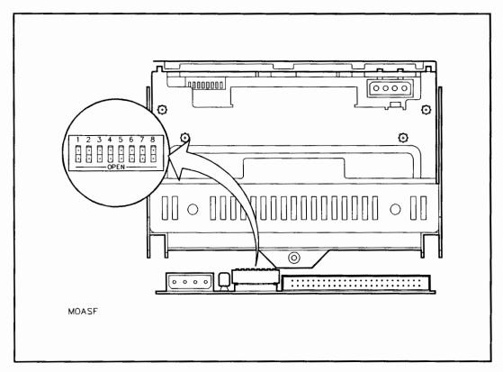
Figure 3-5. Rewritable Optical Disk Drive Address Switch
