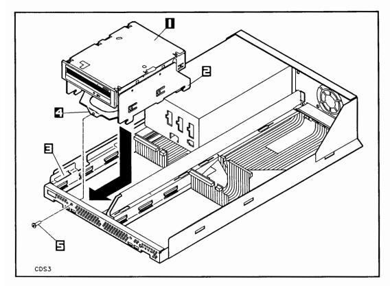
Figure 4-11. Installing a CD-ROM Drive
