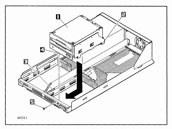
Figure 3-14. Installing the Rewritable Optical Disk Drive
