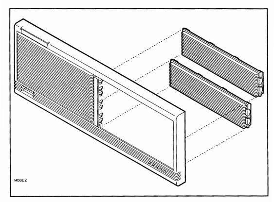
Figure 3-7. Removing the Front Panel Bezels
