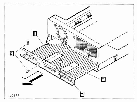
Figure 3-9. Removing the BEND/flex Cable
