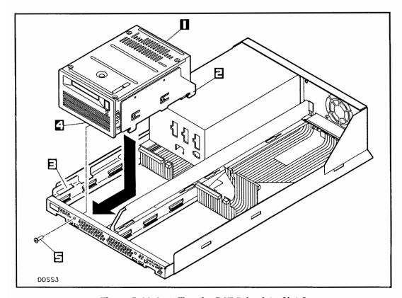
Figure 5-11. Installing the DAT Drive into Slot 3
