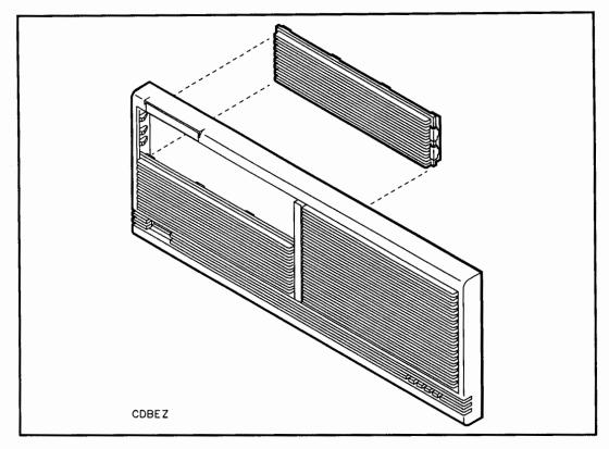
Figure 4-7. Removing a Front Panel Bezel
