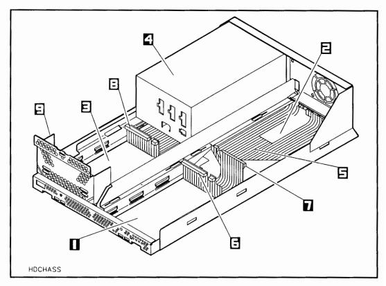
Figure 3-8. Mass Storage System Chassis
