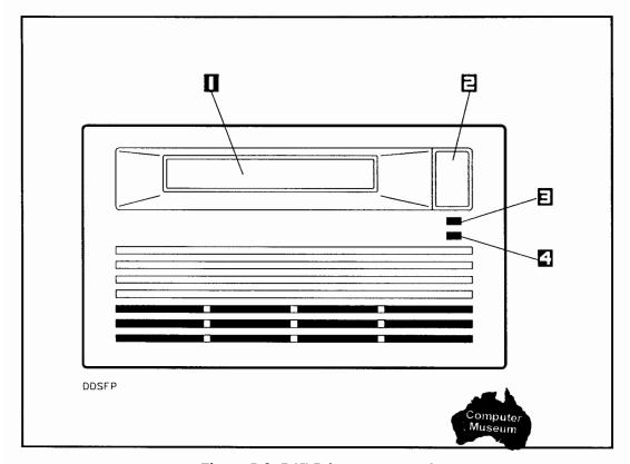
Figure 5-3. DAT Drive Front Panel
