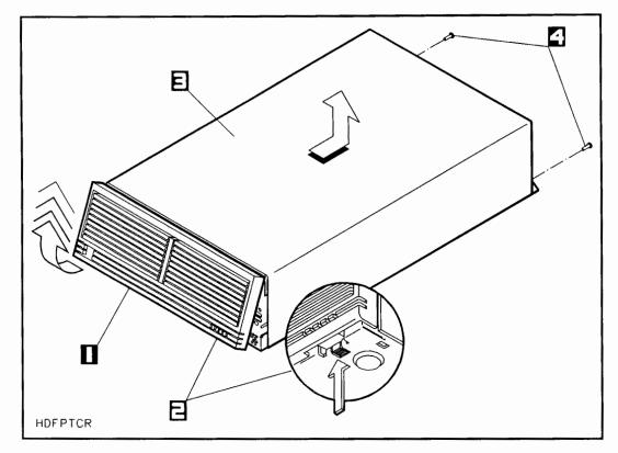
Figure 2-3. Removing the Front Panel and Top Cover
