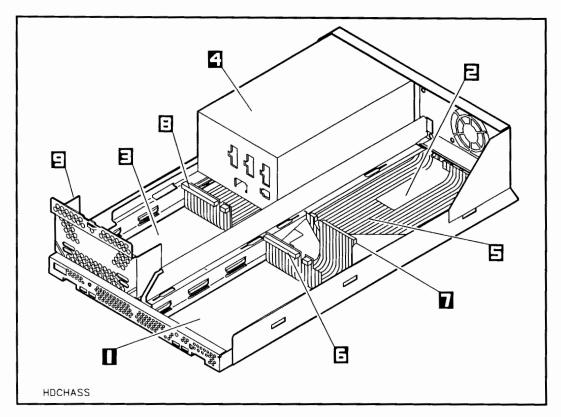
Figure 2-4. Mass Storage System Chassis
