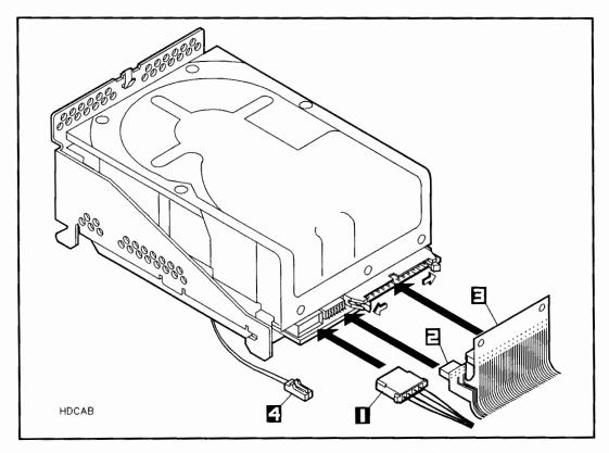
Figure 2-10. Connecting Cables to the Hard Disk Drive
