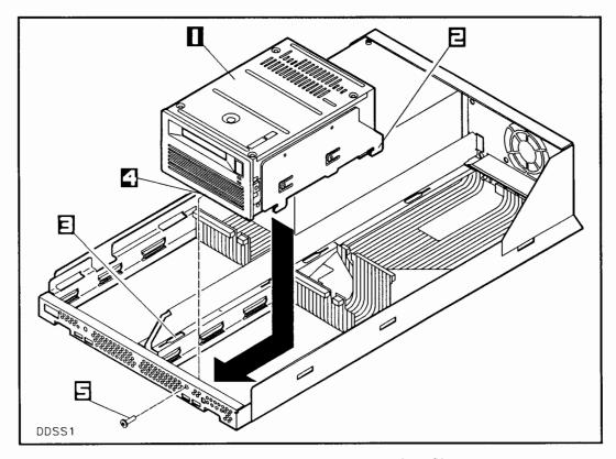
Figure 5-10. Installing the DAT Drive into Slot 1
