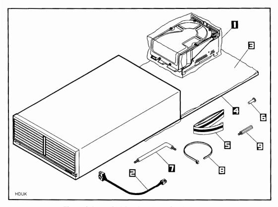
Figure 2-2. Hard Disk Drive Upgrade Kit Contents
