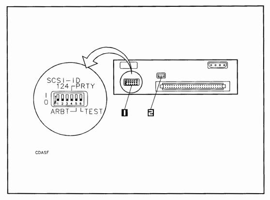
Figure 4-5. CD-ROM Drive Rear Panel Switches
