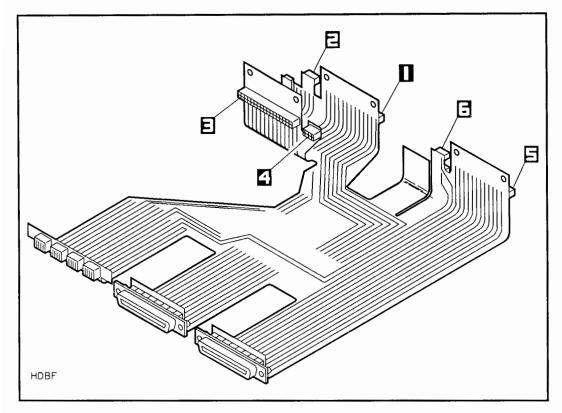
Figure 2-9. BEND/flex Cable Connectors
