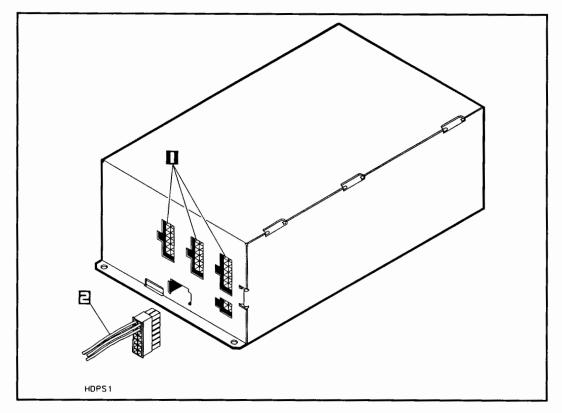
Figure 3-13. Connecting the DC Power Cable
