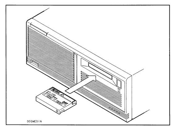
Figure 5-2. Inserting a DAT Cassette
