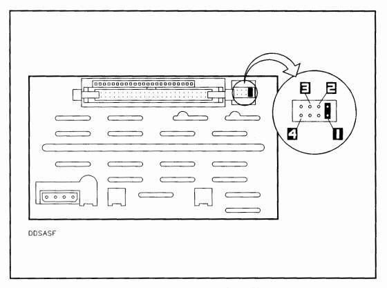
Figure 5-5. DAT Drive Address Pins
