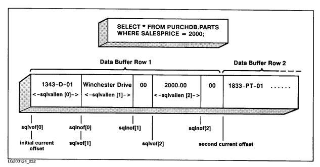
Figure 8-6. Parsing the Data Buffer in cex10a
