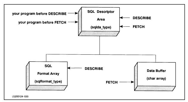
Figure 8-4. Dynamic Query Data Structures and Data Assignment
