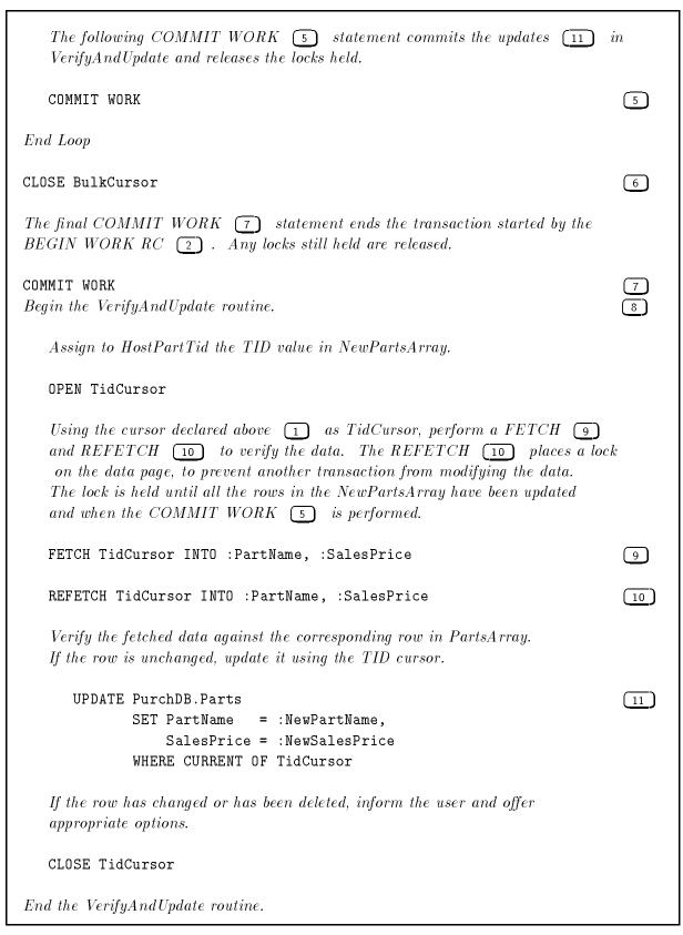
Figure 11-3. Using TID Access to Reduce Commit Overhead (2 of 2)
