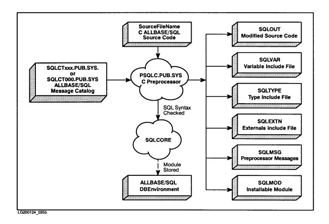
Figure 2-5. Full Preprocessing Mode Input and Output
