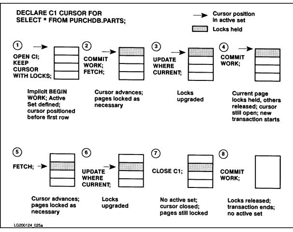
Figure 8-2 shows the effect of the KEEP CURSOR WITH LOCKS.
