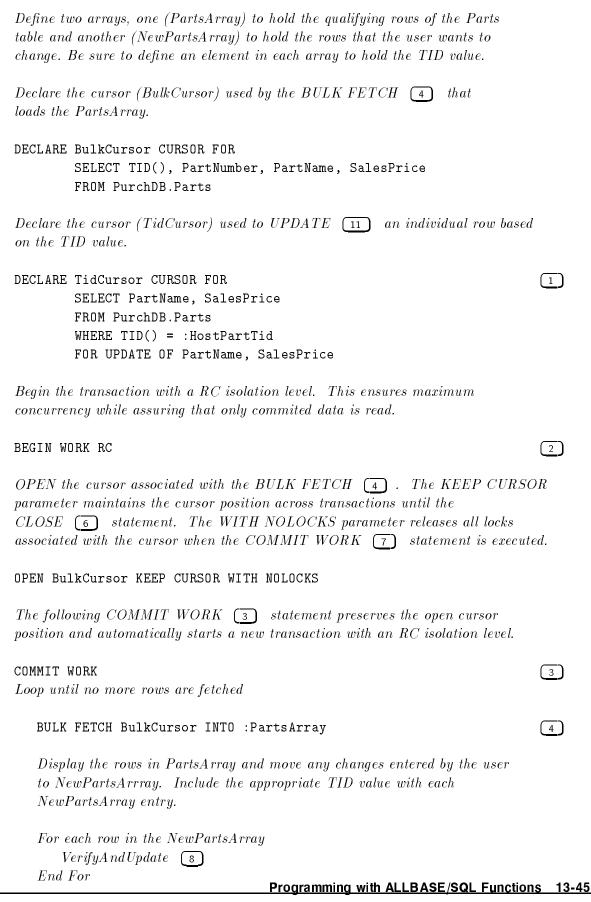
Figure 13-4. Using TID Access to Reduce Commit Overhead
