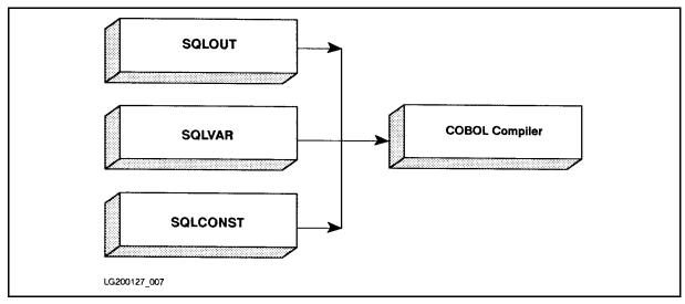
Figure 2-3. Compiling Preprocessor Output
