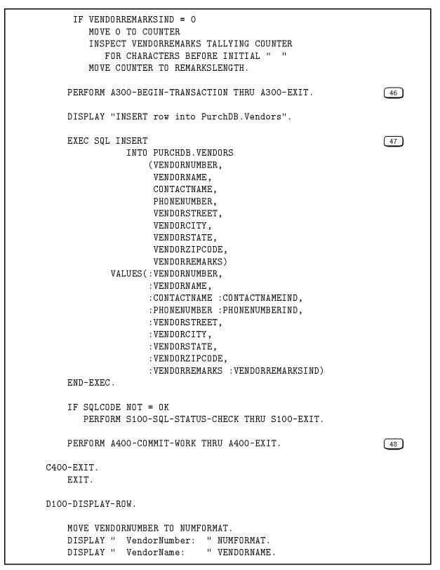
Figure 7-3. Using INSERT, UPDATE, SELECT and DELETE (page 12 of 14)
