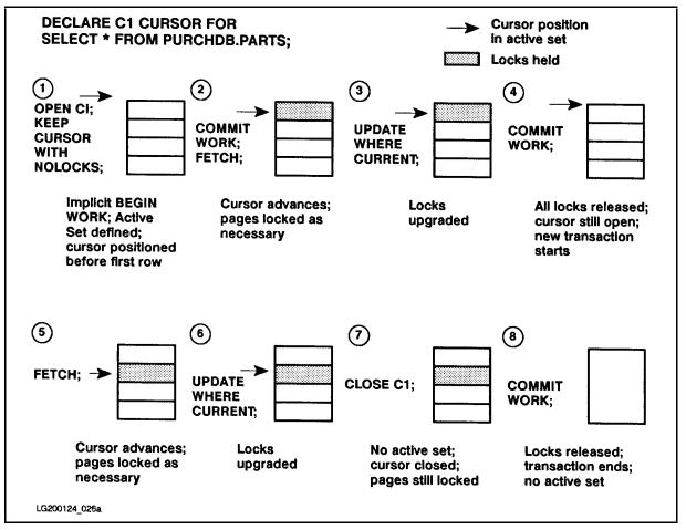
Figure 8-3. Cursor Operation Using KEEP CURSOR WITH NOLOCKS
