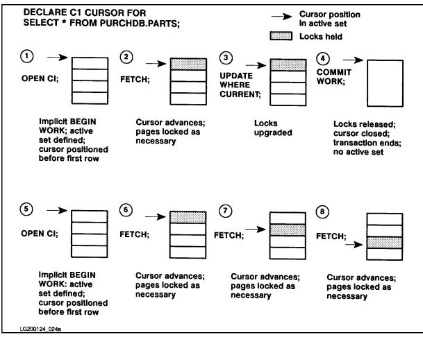
Figure 8-1. Cursor Operation without the KEEP CURSOR Feature
