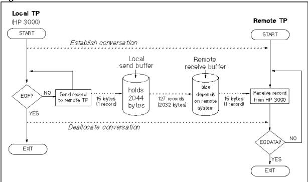
Figure 6-1 Send and Receive Buffers
