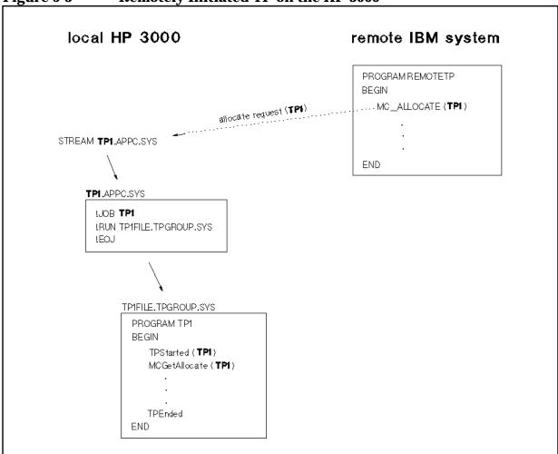
Figure 5-3 Remotely Initiated TP on the HP 3000
