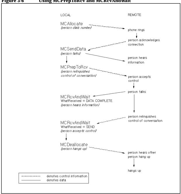
Figure 3-6 Using MCPrepToRcv and MCRcvAndWait
