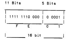
2. Take the bank number in the lower 5 bits and place it in a temporary register. Zero fill the lower 5 bits overwritting the bank #.
