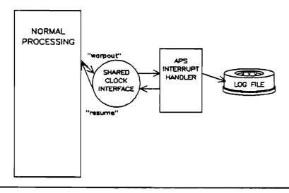
The APS/3000 analyzer module can then analyze the log file and produce reports showing where it found the CPU.
