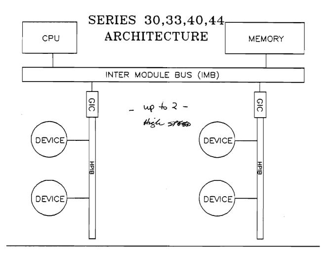
This is the basic HPIB architecture. It form the basis for ALL the HPIB systems. Point out to the students that the series 39,40SX, 42, and 48's also use this architecture.
