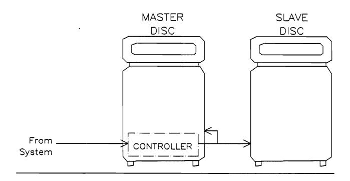
This slide indicates how slave discs are used. A single disc controller can only TRANSFER data to one disc drive at a time. Unless some additional tricks are used then adding a SLAVE disc to a system will not increase disc performance substantially. (Neglecting the effect of minimizing seek times on single disc systems).
