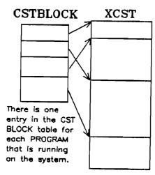
The XCST contains blocks of CST entries, one for each program file that is being run on the system.
