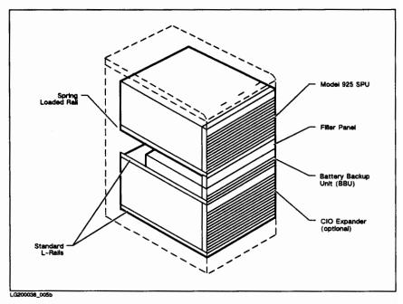
Figure 2-4. Model 925 System in a Small Cabinet
