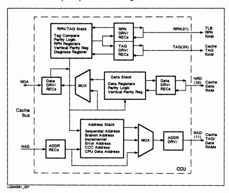
Figure 9-6. 825/925 CCU Chip Simplified Block Diagram
