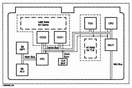
Figure 9-3. 835 Processor Card Block Diagram
