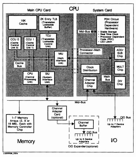
Figure 9-1. 825/925 System Block Diagram
