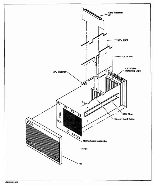
Figure 8-1. SPU Exploded View
