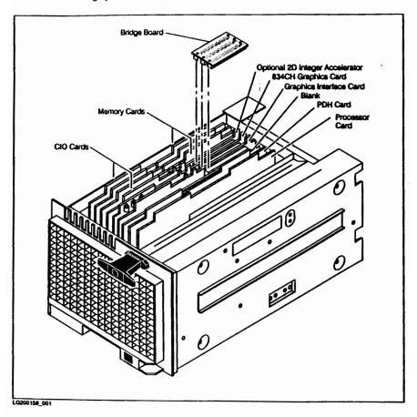
Figure B-2. Model 834CH SPU Orientation
