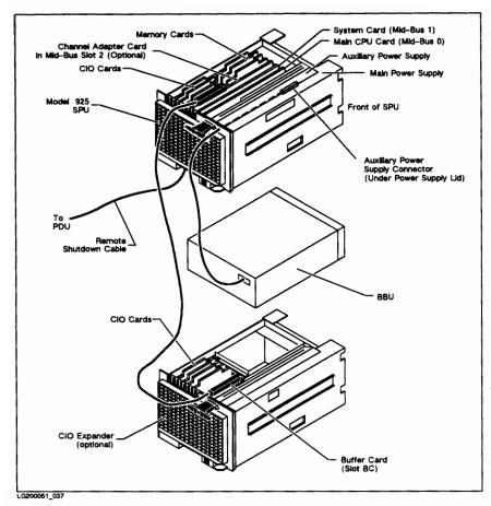
Figure 1-5. Model 925 Orientation
