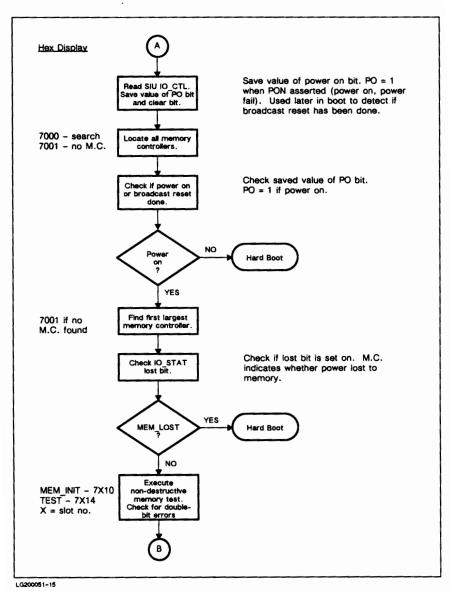
Figure 4-12. Selftest Detailed Flowchart (cont'd)
