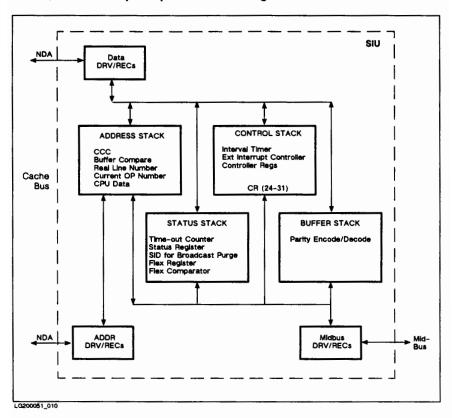
Figure 9-9. 825/925 SiU Chip Simplified Block Diagram
