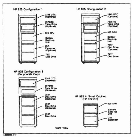
Figure 2-1. Model 925 Configurations
