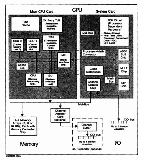
Figure 1-1. 825 and 925 System Block Diagram
