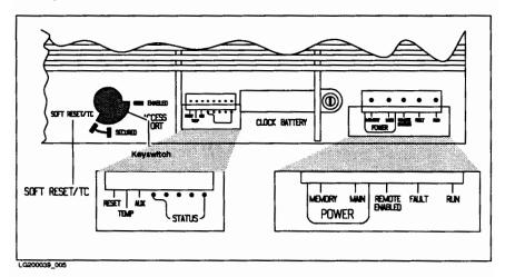
Figure 4-3. Front Panel Layout
