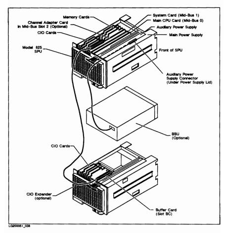
Figure 1-3. Model 825 Orientation
