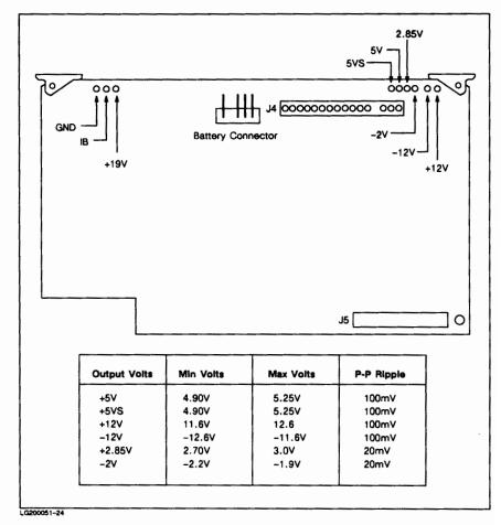
Figure 4-9. Test Points on the Auxiliary Power Supply
