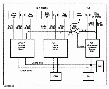
Figure 9-2. 825/925 Cache Subsystem Block Diagram
