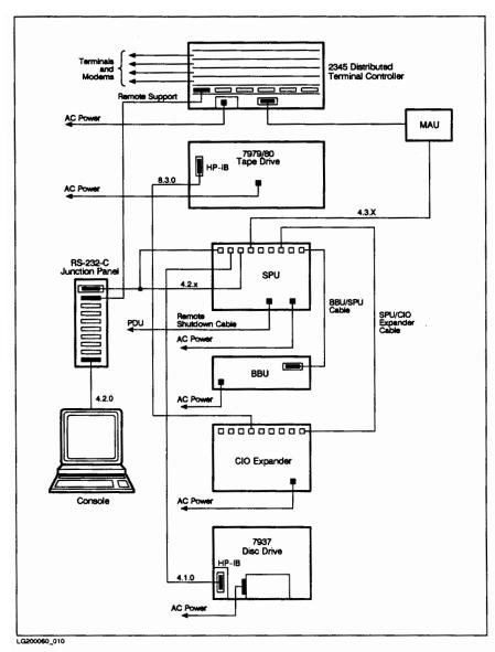
Figure 2-3. Typical Cable Connections for Configuration 1 (Sample)
