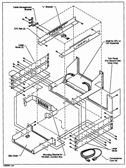
Figure 8-6. Mounting Hardware of the A1001A Large Cabinet
