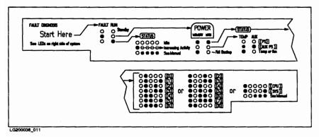
Figure 4-4. Fault Diagnosis Flowchart
