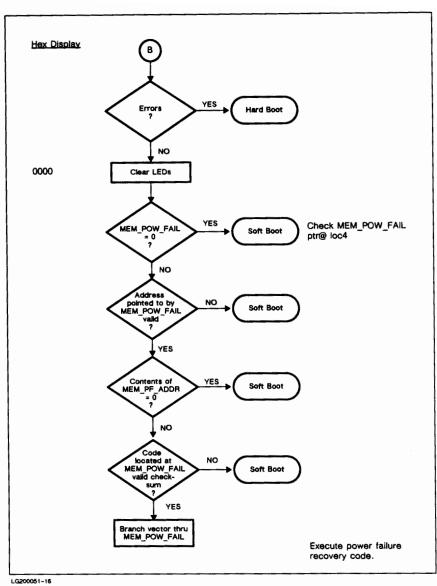
Figure 4-13. Selftest Detailed Flowchart (cont'd)
