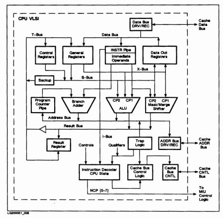
Figure 9-8. 825/925 CPU Chip Simplified Block Diagram
