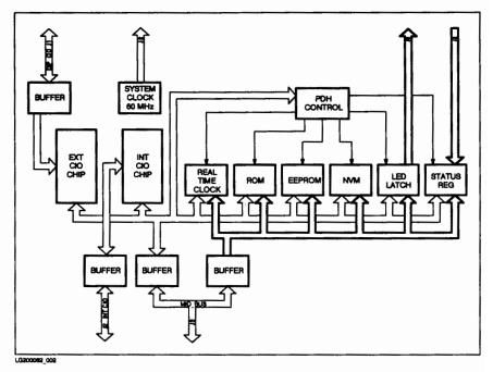
Figure 9-4. 835 PDH Card Block Diagram
