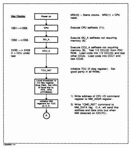
Figure 4-11. Selftest Detailed Flowchart
