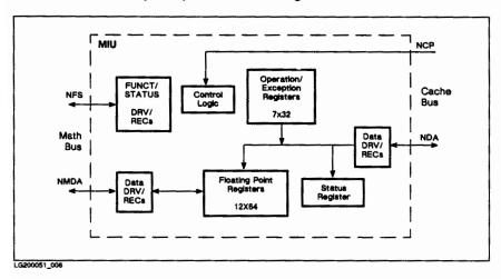
Figure 9-5. 825/925 MIU Chip Simplified Block Diagram
