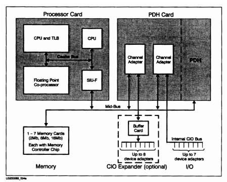
Figure 1-2. 835 System Block Diagram
