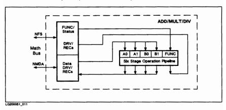
Figure 9-10. 825/925 Math Chip Simplified Block Diagram
