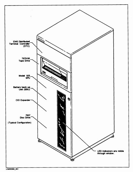
Figure 2-2. Model 925 System in a Large Cabinet
