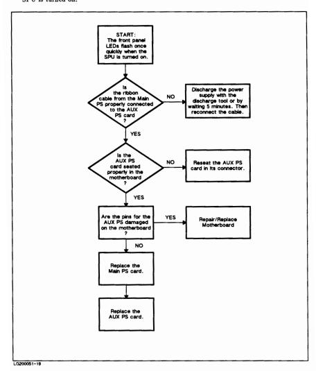
Figure 4-8. Troubleshooting when LEDs Flash Once Quickly
