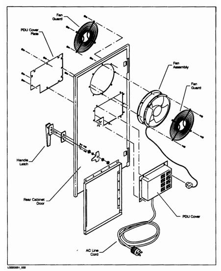
Figure 8-7. Rear Door of the A1001A Large Cabinet
