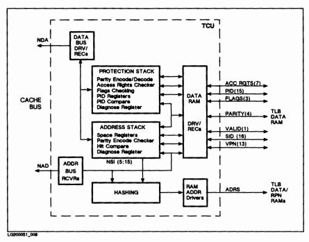
Figure 9-7. 825/925 TCU Chip Simplified Block Diagram
