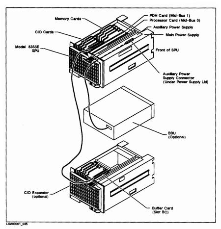
Figure 1-4. Model 835SE Orientation
