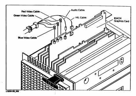
Figure B-3. Model 834CH Graphics Card Connectors
