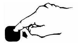
Continue key: Press to clear errors and resume printing. (Option 200/210 also allows reset when offline – press key and hold for 2 seconds).
