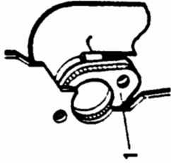
Figure 28. Cleaner Station Vacuum Connection Seal
