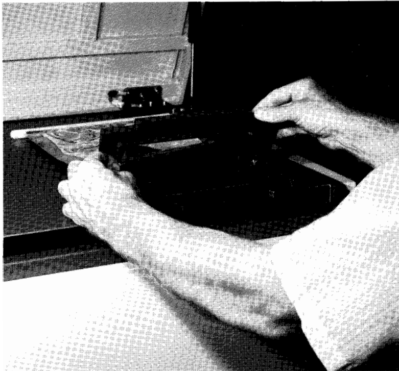
Figure 3-18. Opening Toner Hopper Lid
