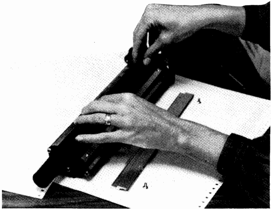
Figure 4-16. Installing New Wiper Blade
