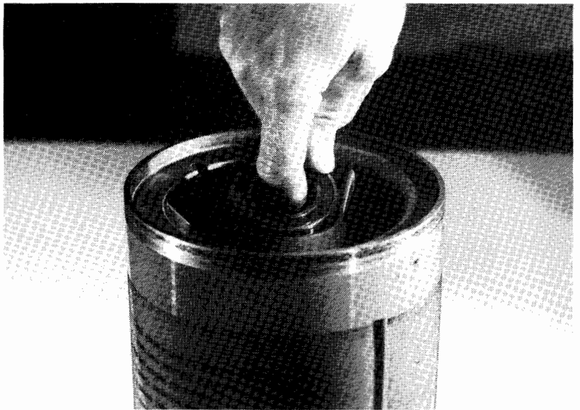
Figure 4-13. Removing Photoconductive Drum Bearing
