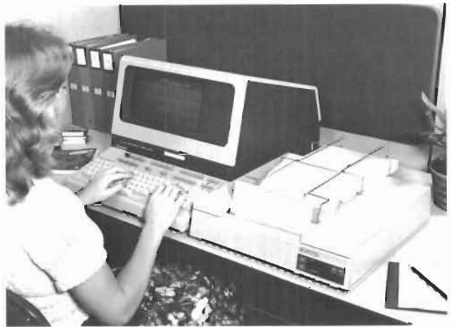
The 2671G and the 2673A copy screen graphics directly from HP 2647A and HP 2648A terminals.
