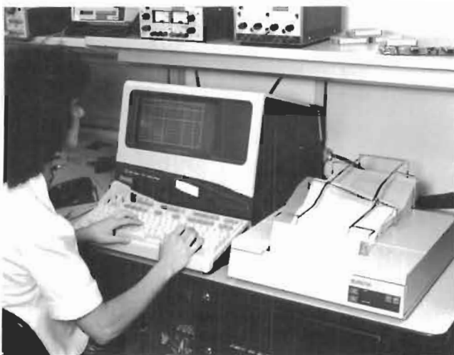
The 2671A's standard forms printing capability is compatible with HP 2640 and HP 2620 series terminals.
