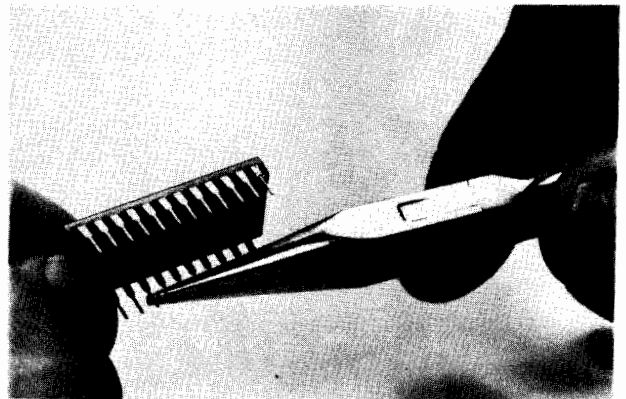
Straightening Bent Pins with Pliers
