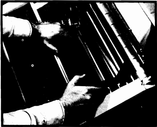
Fig. 6. Full-width ribbon cartridge is easily replaced.
