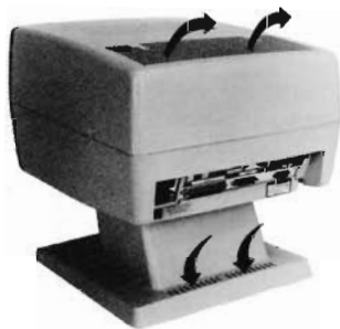
Figure 2-2. Cooling Airflow Through the Terminal
