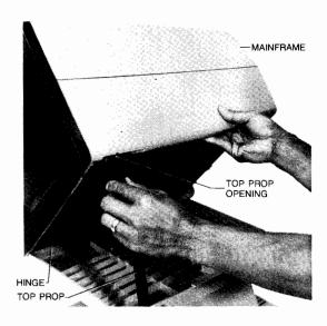
Figure 2-3. Freeing Mainframe from the Top Prop
