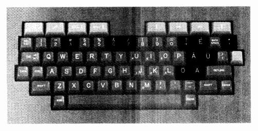
Figure 7-19. Swedish/Finnish Keyboard, Unique Keys
