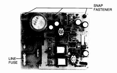
Figure 7-8. Power Supply PCA (2621A)
