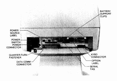
Figure 2-2. Terminal Rear View
