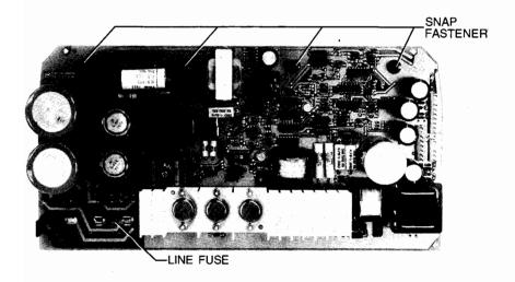
Figure 7-9. Power Supply PCA (2621P)
