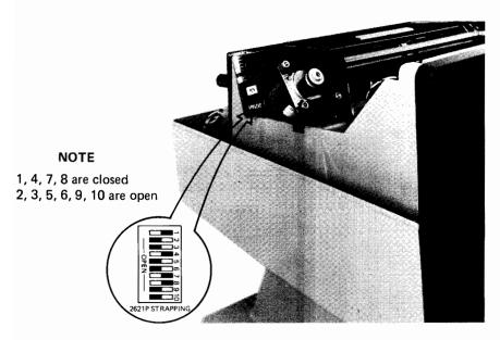
Figure 3-3A. TPM Configuration and Location (TPM PCA Part No. 02670-60050 Standard Terminal)
