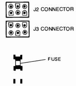
On the 2621P only the fuse position is changed to match the source voltage. The X1 socket is used for voltages between 220 and 240 volts. The X2 socket is used for voltages between 100 and 120 volts.
