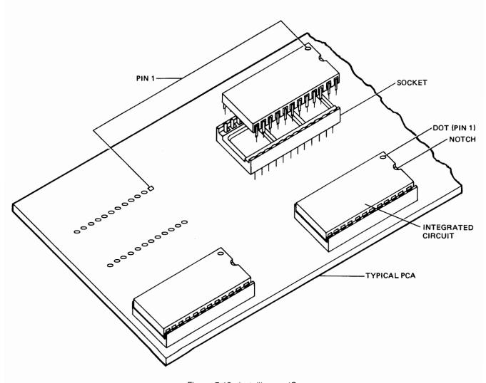
Figure 7-12. Installing an IC
