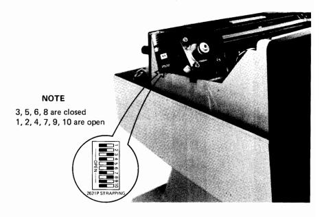
Figure 3-3B. TPM Configuration and Location (TPM PCA Part No. 02670-60050 National Option)
