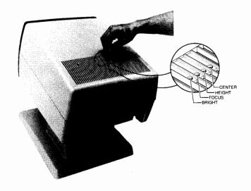
Figure 5-3. Location of Four Raster Adjustments (CENTER, HEIGHT, FOCUS, and BRIGHT)
