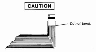
When replacing the print head assembly do not bend the flex cable where it connects to the print head.
