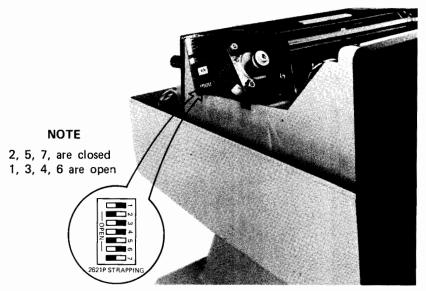
Figure 3-3. TPM Configuration and Location (TPM PCA Part No. 02670-60001)
