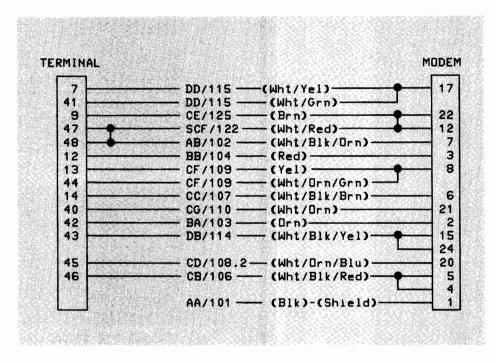
Figure 2-10. 13222W (HP 300) Cable Wiring
