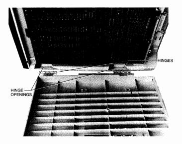
Figure 2-4. Mating the Hinges to the Hinge Openings
