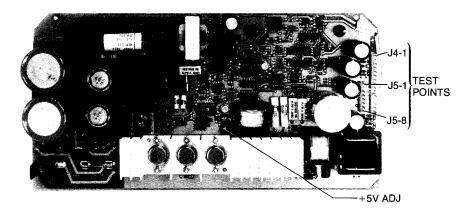
Figure 5-2. 2621P Terminal Test Points and +5V Adjustment Locations
