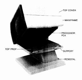
Figure 2-1. Terminal in Half-Open Position
