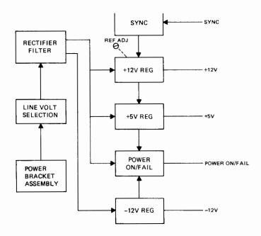
Figure 8-5. 2621A Power Supply, Simplified Block Diagram
