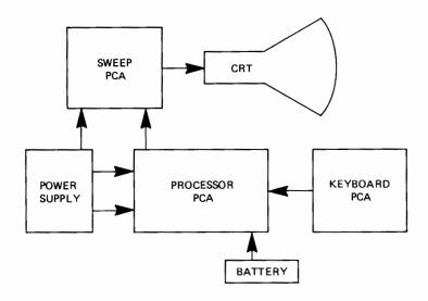
Figure 8-1. 2621A Simplified Block Diagram
