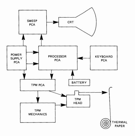
Figure 8-2. 2621P Simplified Block Diagram
