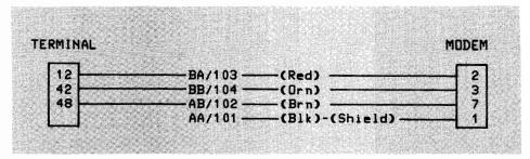
Figure 2-11. 13222Y (Three Wire/Male) Cable Wiring
