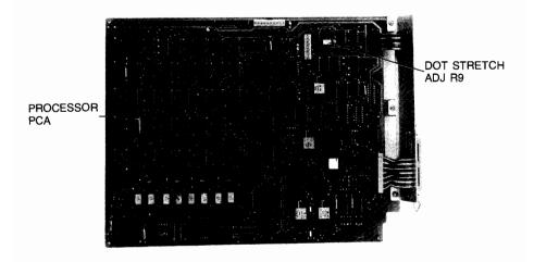
Figure 5-5. Dot Stretch Adjustment Location
