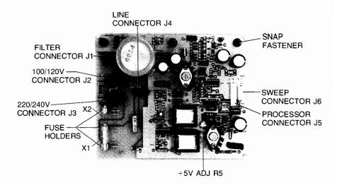
Figure 2-5. 2621A Power Supply PCA
