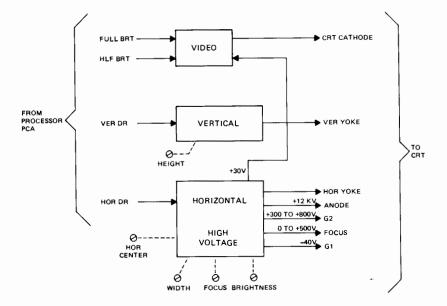
Figure 8-4. Sweep PCA, Simplified Block Diagram
