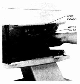
Figure 5-4. Location of Raster Width Adjustment and Yoke Collar
