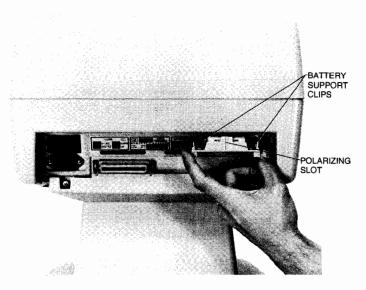
Figure 4-1. Battery Removal
