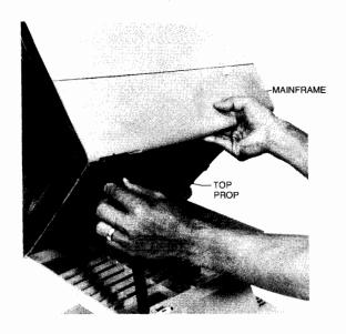
Figure 7-3. Terminal Set to the Half-Open Position
