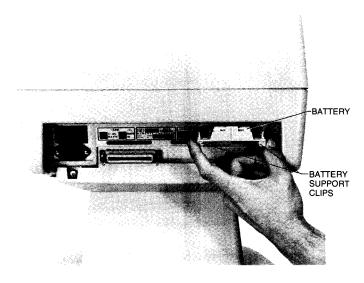
Figure 7-11. Battery Removal
