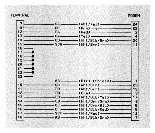
Figure 2-9. 13222N (U.S. Modem) Cable Wiring
