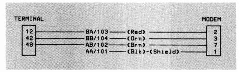
Figure 2-12. 13222Z (Three Wire/Female) Cable Wiring
