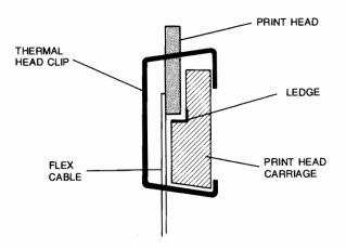
Figure 7-13D. Ledge Inside Print Head Carriage
