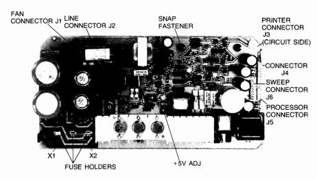
Figure 2-6. 2621P Power Supply PCA
