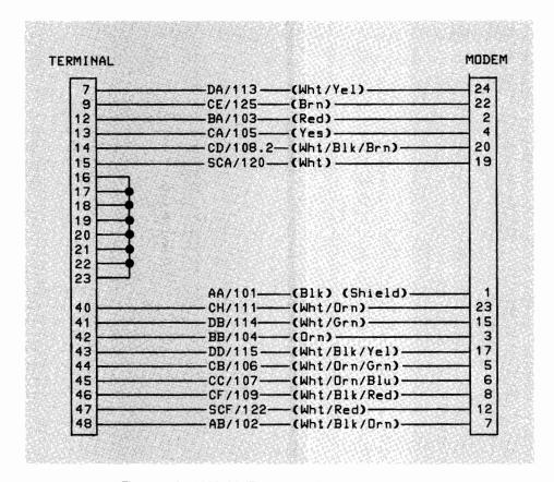
Figure 2-8. 13222M (European Modem) Cable Wiring
