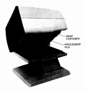
Figure 7-6. Processor PCA Removal
