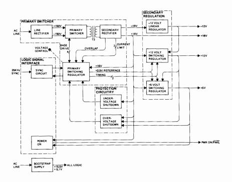
Figure 8-6. 2621P Power Supply, Simplified Block Diagram
