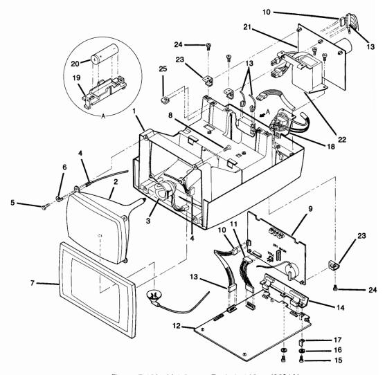
Figure 7-16A. Mainframe, Exploded View (2621A)
