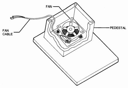
Figure 7-5. Fan Removal (2621P)
