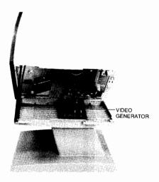
Figure 6-4. Video Generator Installed in Place of the Processor PCA
