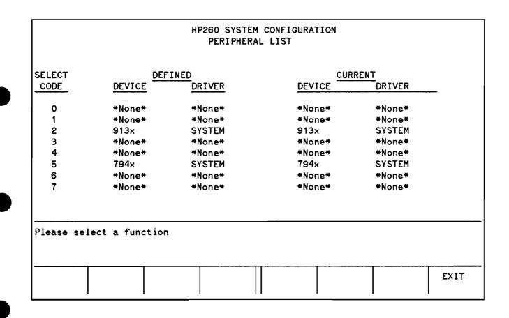
The device address assigned to each system I/O driver cannot be changed. To change the device address assigned to a non-standard I/O driver, first press EXIT to return to the initial menu. Then select function 4 from the initial CONFIG menu to run the peripheral edit routine.
