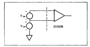
EXAMPLE: On the ±250 mV range, the maximum differential input input allowed is 250 mV, therefore V<sub>crr</sub>(maximum) =: 10-250 mV = 9.750V
