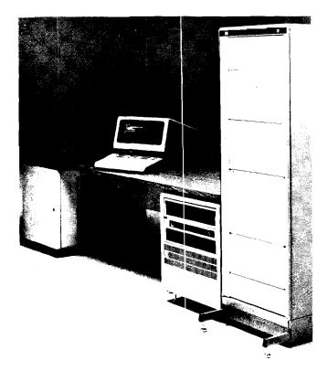
2250R — 56" racked system (at right, shown with HP 1000 Model 45 computer system) including terminations for field wiring. Can be expanded to 2048 points for application in lab facilities, complex product tests or supervisory control.
