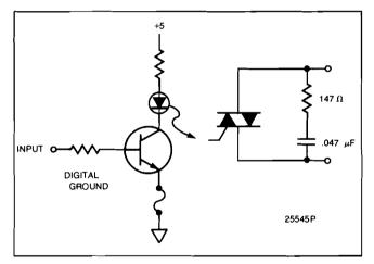
Maximum holding current: 1 mA without snubber; 4 mA with snubber.
