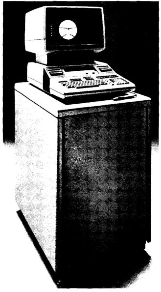
**2250M** — 30" racked system for smaller test and control applications requiring up to 256 measurement points. Field wiring terminations can be installed permanently or cable harnesses may be connected temporarily for roll-around use.
