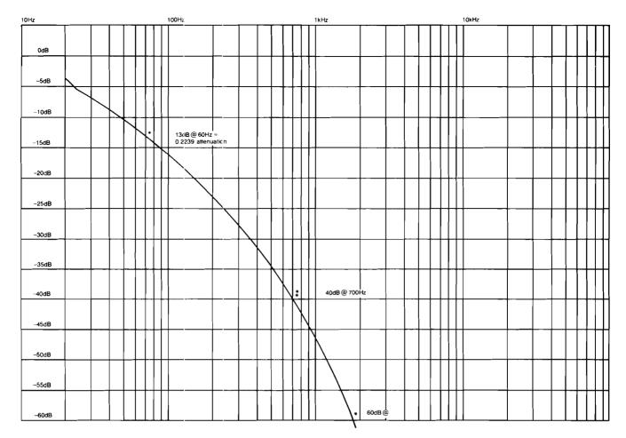
25540C and 25540D Analog SCMs Filter Frequency Characteristics
