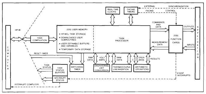
ous buffered data gathering and transmission. Multiple tasks may be compiled and stored locally for later execution. Tasks may be scheduled upon interrupt from a function card or on command from another request or task. Other capabilities include history data acquisition, analog offset correction, time-of-day clock, and built-in processor self-test.
