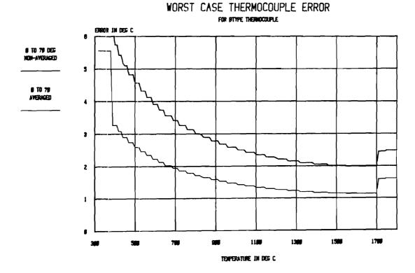
WORST CASE THERMOCOUPLE ERROR FOR & TYPE THERMOCOUPLE
