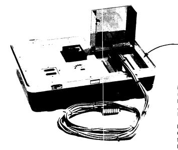
DIAGNOSTIC UNIT IDENTIFIES THE BOARD FROM A RESISTOR VALUE AND THEN TESTS IT FROM THE CARD EDGE USING THE 2250 PROCESSOR. FAULTY BOARDS ARE QUICKLY IDENTIFIED WITH A MINIMUM OF EXPERTISE OR EQUIPMENT.
