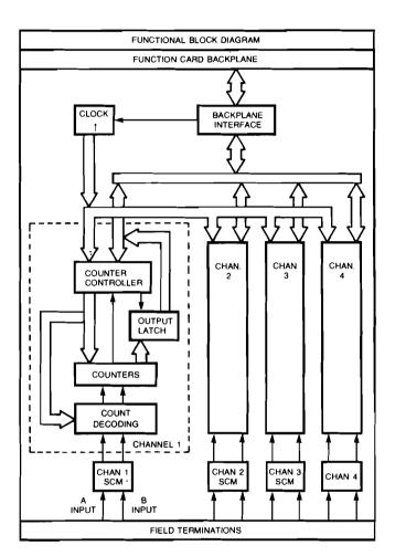
Each channel uses one signal conditioning module (SCM) for its A and B inputs. This allows each channel to interface to a different level or type of signal for maximum flexibility. Channels may be programmed to respond to falling or rising edges. In up-down count mode, one of three types of input can be selected: up counts and down counts, count and direction, or quadrature.
