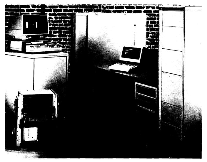
The 2250 family of products consists of integrated systems, processor units, function cards, function card frames, and signal conditioning modules. All 2250 systems offer completely integrated products in both rack-mount and NEMA\* cabinets. Frames, cards, and cables are all installed and tested in system configurations. The three configurations are the 2250M/N/R.
