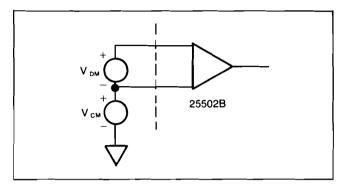
Example: With a common mode voltage of +4 volts, the maximum differential voltage that can be measured would be ±6 volts.
