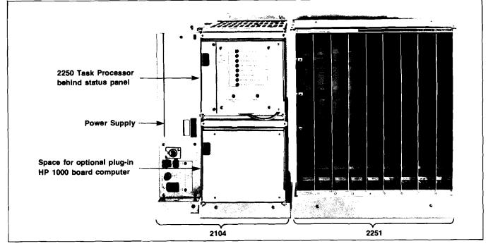
The 2104A Processor Unit has a 4 card microcomputer to run MCL/50 and down-loaded Fortran tasks: a CPU, a ROM/RAM memory card, an HP-IE interface and an interface to the 2250 Function card backplane.
