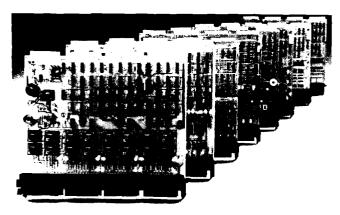
The Function Card family provides the measurement and control functions: analog or digital, input or output. Each card handles up to 32 channels of data, where a channel is one analog signal or one digital bit.
