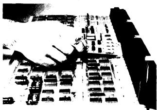
Signal Conditioning Modules (SCM) provide the final conversion of electrical levels to match your sensors and actuators. They plug onto the Function Cards in channel groups, and provide filtering, isolation, and voltage level conversion as needed.
