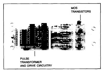
Maximum rise time ( $\mu$ sec): 25; VDD = 60V, R(load) = 200 ohms Maximum fall time ( $\mu$ sec): 2; VDD = 60V, R(load) = 200 ohms Maximum turn-on delay ( $\mu$ sec): 2 Maximum turn-off delay ( $\mu$ sec): 30
