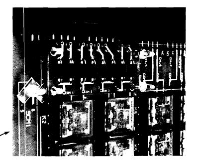
PLUG-ON SIGNAL CONDITIONING MODULES CONFIGURE THE VOLTAGE LEVELS AND FILTER CHARACTERISTICS. THEY ARE HELD BY NYLON STANDOFFS AND HAVE GOLD-TO-GOLD GAS TIGHT CONTACTS. BECAUSE THE FUNCTION CAFID HAS NO SOLDERED-IN JUMPERS OR COMPONENTS, IT CAN BE SERVICED BY BOARD EXCHANGE.
