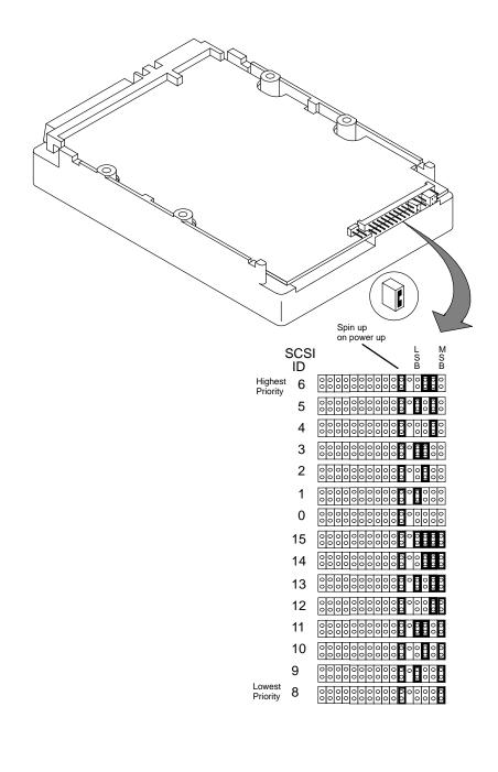
Seagate ST32171WD and ST34371WD Disk Drive Jumpers
