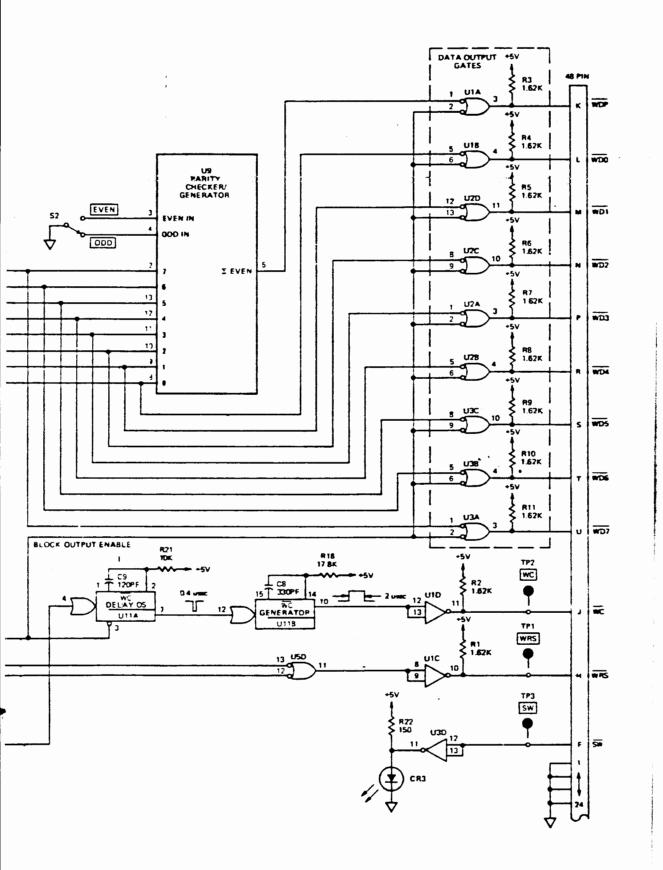
Figure 5-6. Main Write Test Board (A1) Component Location Diagram, Signal Summary Table, and Schematic Diagram
