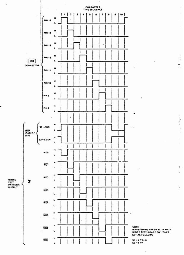
Figure 5-7. Write Program 1 Test Board (A2) Parts Location, Schematic and Waveform Diagrams
