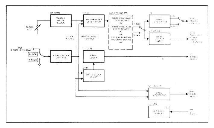
Figure 4-3. Write Test Accessory Simplified Logic Diagram
