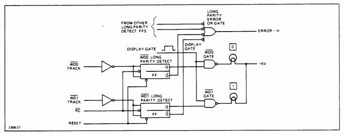
Figure 4-6. Simplified Longitudinal Parity Error Circuits
