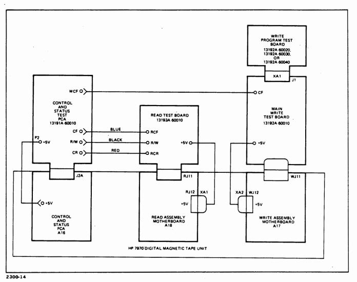
Figure 2-2. Test Accessory Interconnection Diagram
