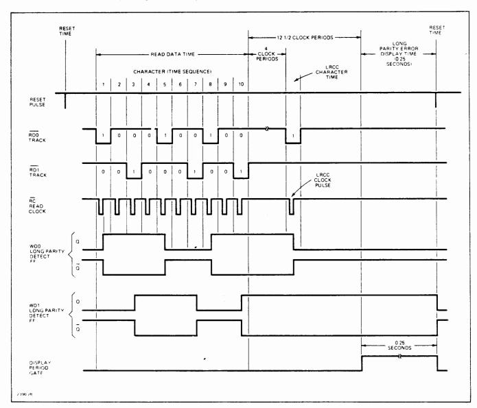
Figure 4-7. Longitudinal Parity Check Waveforms
