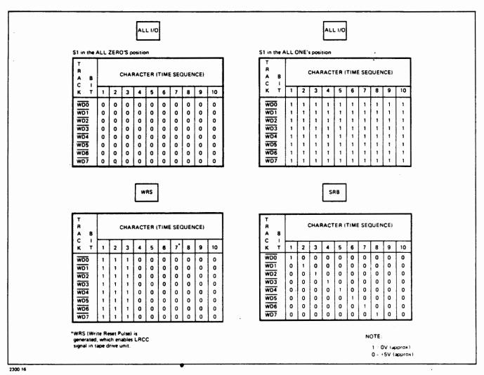
Figure 3-4. Write Test Accessory Data Program 1 Output Pattern
