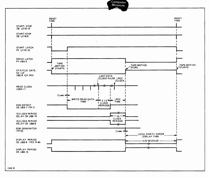
Figure 4-9. Read Test PCA R/W Waveforms
