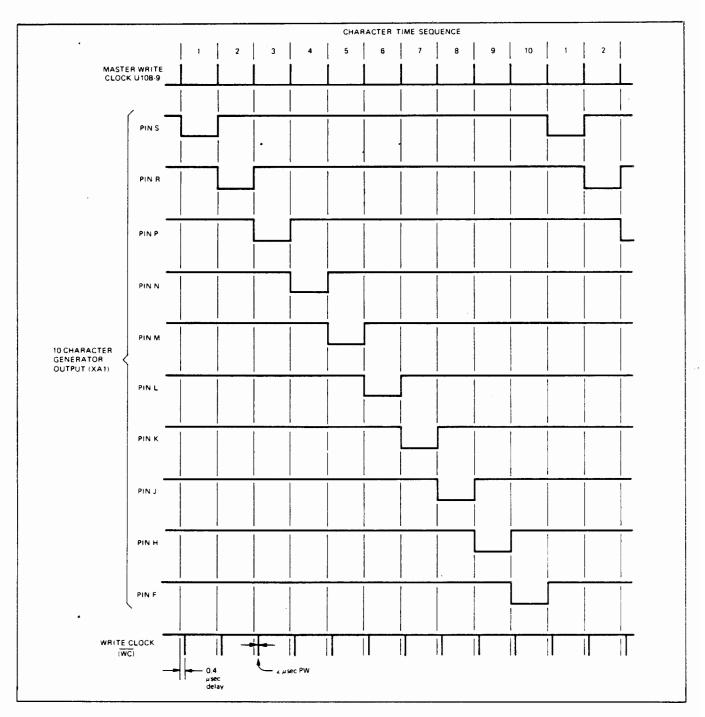
Figure 4-4. Ten-Character Generator and Write Clock (WC) Output in the X TALK (Continuous) Mode
