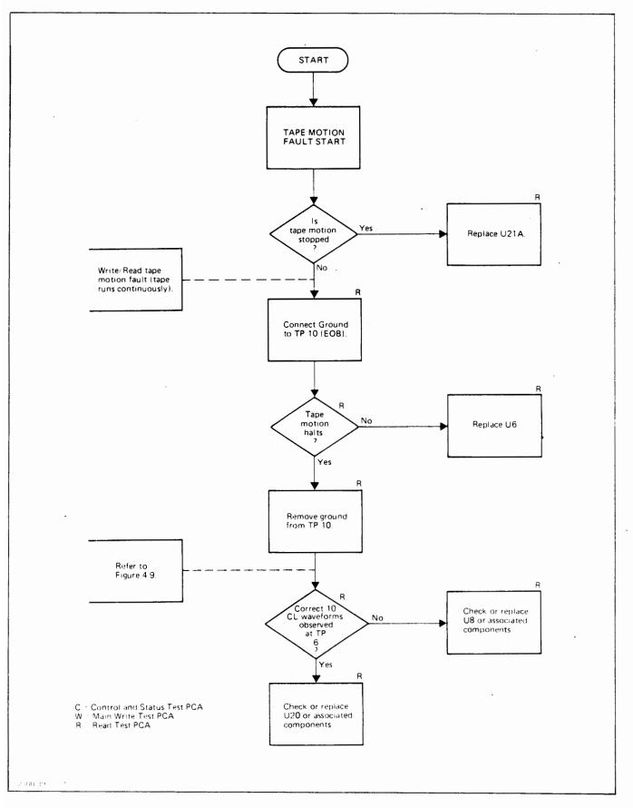
Figure 5-1. Tape Motion Fault Troubleshooting Diagram
