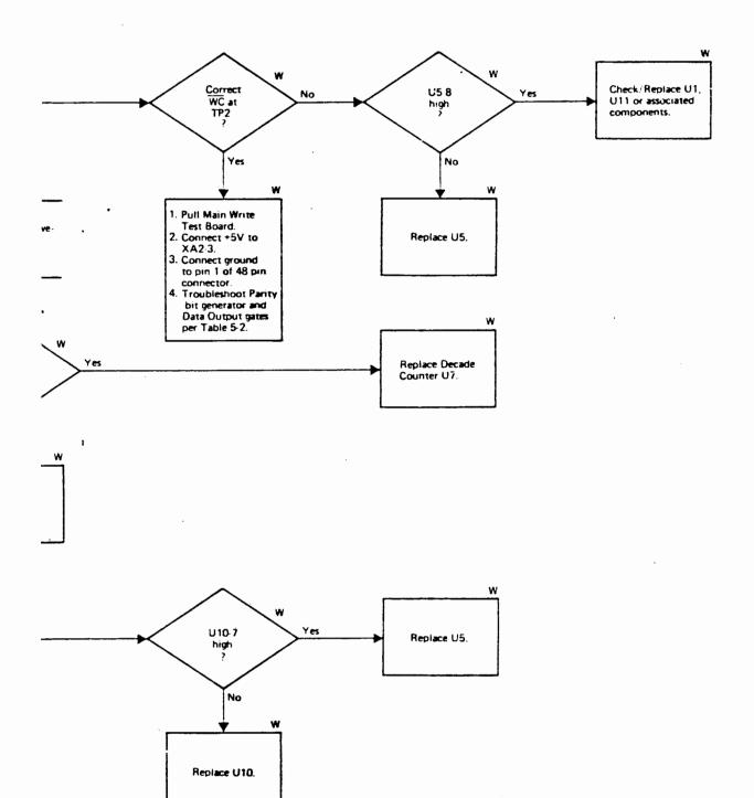
Figure 5-2. Write Data Fault Troubleshooting Diagram
