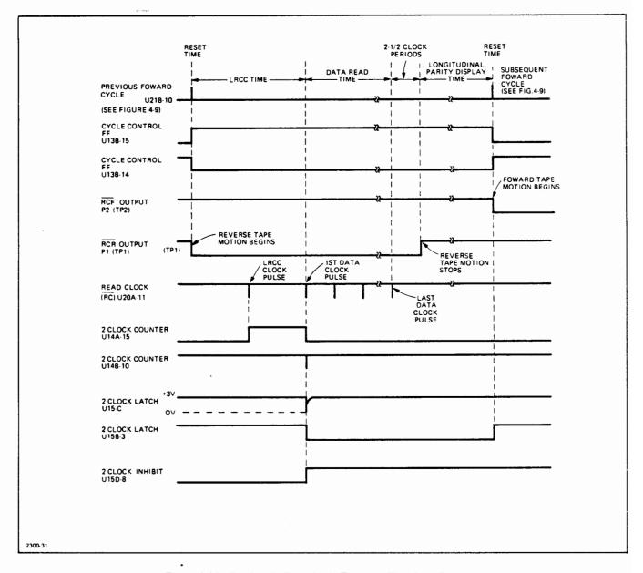
Figure 4-10. Read-Only Test, Cycle Function Waveform Diagram
