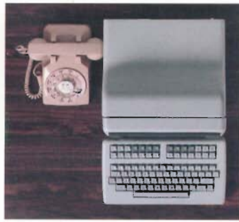
A personal computer designed to fit on your desk... the HP 120 computer electronics, display, keyboard and disc drives take up only 1.7 square feet of desk space.
