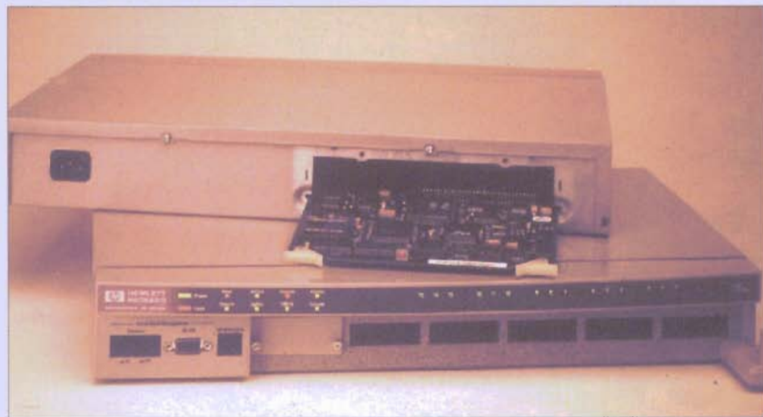
HP's AdvanceStack 100VG Hub-15 is key to the 100VG design, providing 15 100Mbps LAN ports, with room for an optional bridge/SNMP module for connection to 10Mbps networks.
