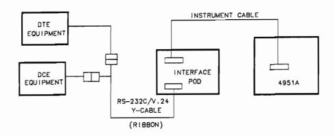
Figure 2-1. Hookup for Line Monitoring
