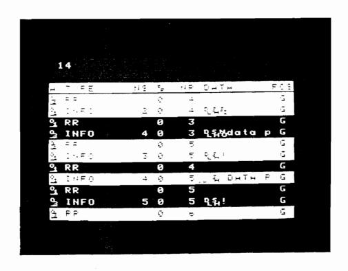
Figure 5-4. X.25 in Frame & Packet Display Format (Examine Data Menu)
