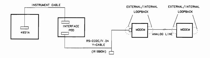
Figure 9-3. Loopback Testing
