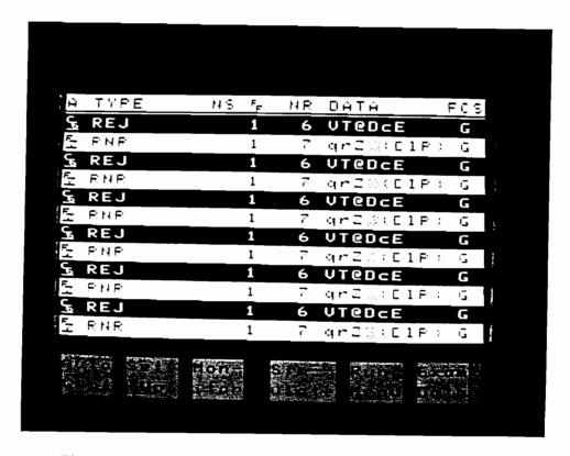
Figure 5-2. HDLC in Frame & Packet Display Format (run-time)
