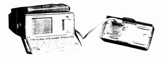
Figure 1-1. The 4951A with Interface Pod
