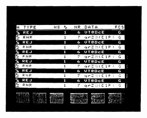
Figure 7-7. Frame & Packet Display Format (See chapters 5 and 8 for definitions)
