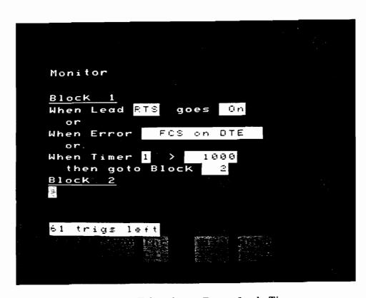
Figure 6-5. Triggering on Errors, Leads, Timers
