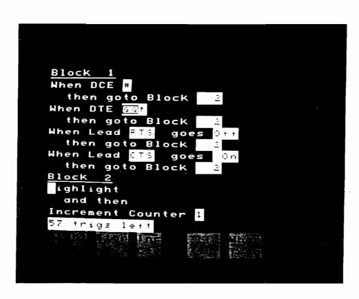
Figure 6-7. Program Producing the Display in Figure 6-6.
