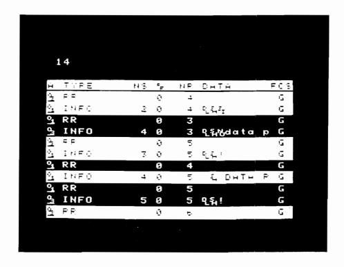
Figure 8-2. Decoding X.25 Packets with Frame & Packet Format
