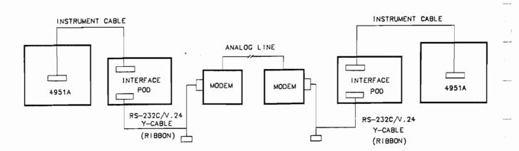
Figure 9-2. End-to-End Testing
