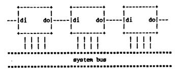
When a chip is unconfigured, it does not occupy address space and its daisy-out is held low. If its daisy-in is low, it will not respond to any CPU instructions. If its daisy-in is high, it will respond to two instructions: C=ID, which returns the chip ID to the CPU (see CHIP ID, below), and CONFIG, which assigns an address to the chip and configures it.
