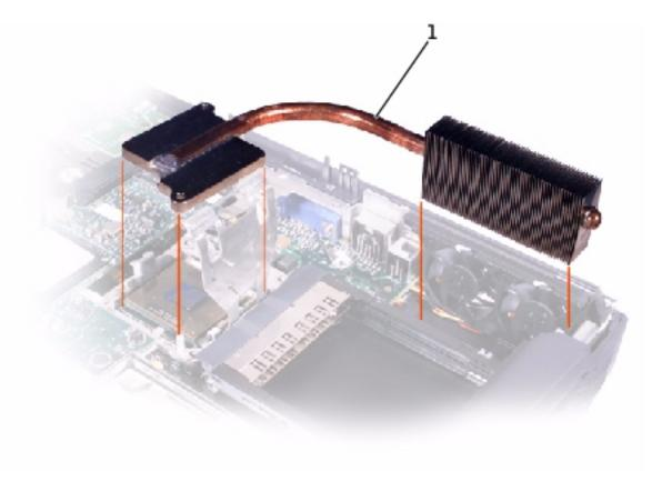
1 microprocessor thermalcooling assembly
