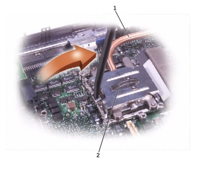
1 microprocessor thermalcooling assembly 2 microprocessor retaining clip
