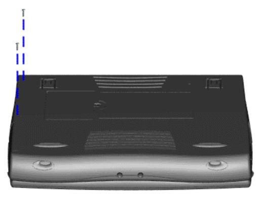
6. Remove two screws from the base enclosure which secure the DVD or CD drive to the chassis.
