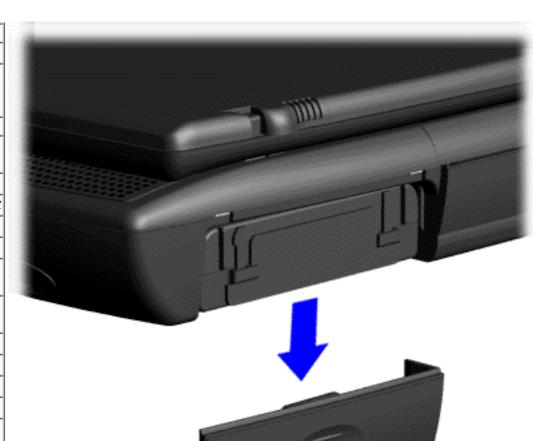
To remove the battery pack, complete the following steps:
